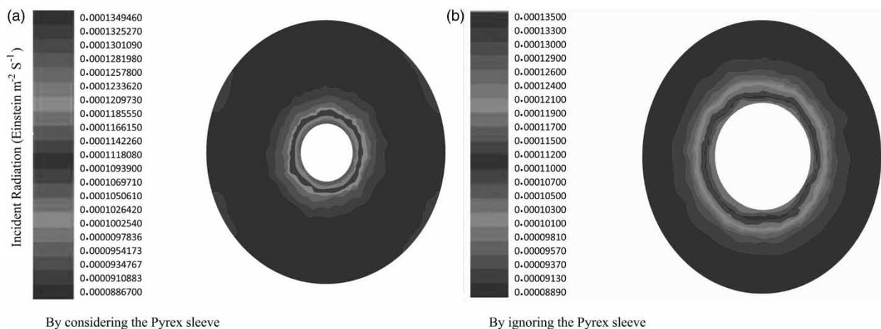
Figure 4 | The effect of the Pyrex sleeve in incident radiation at the catalyst concentration of 0.05 g/l.
