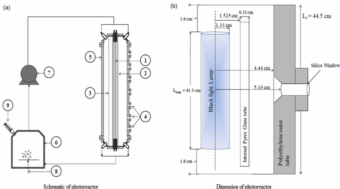
Figure 1 | The photoreactor (Moreira del Rio 2011).
