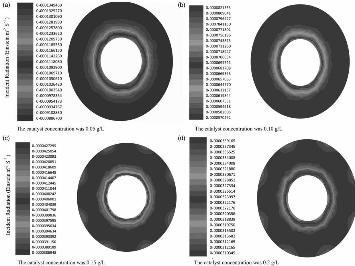
Figure 5 | The incident radiation at various concentrations of the catalyst.
