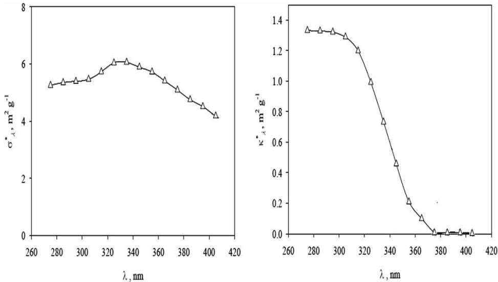
**Figure 3** | Specific scattering and absorption coefficients for TiO<sub>2</sub>-DP25 at wavelength of  $\lambda$  (Romero et al. 2003).
