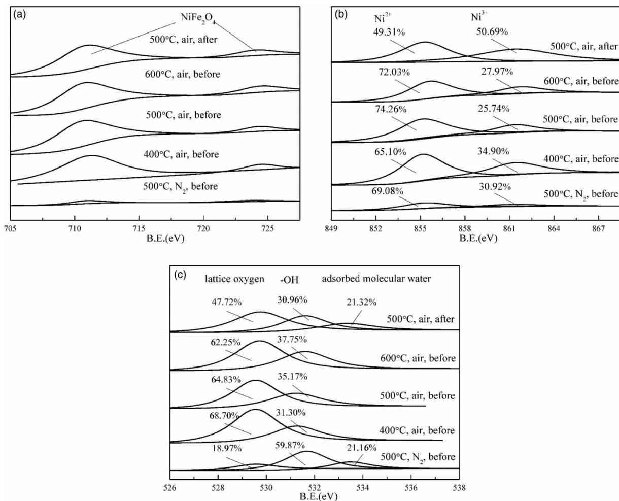
Figure 1 | XPS spectra of different catalysts before and after experiments: (a) Fe, (b) Ni, (c) O.
