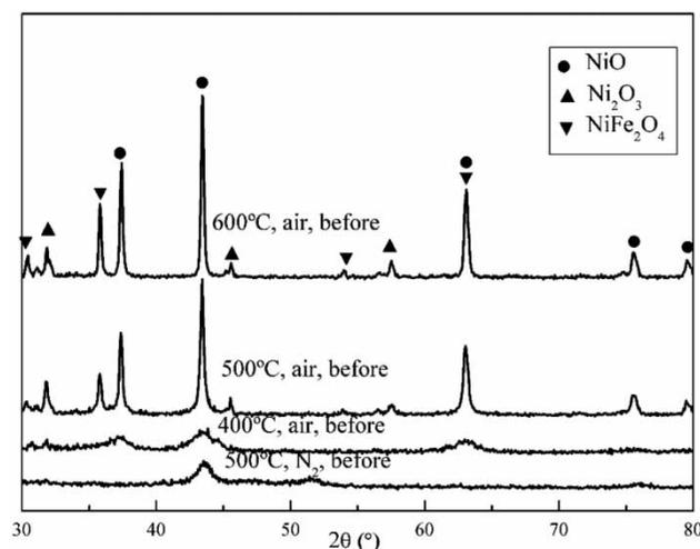
Figure 3 | XRD patterns of different catalysts before and after experiments.
