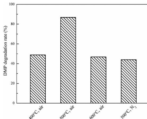
**Figure 5** | DMP degradation rates with different catalysts.
