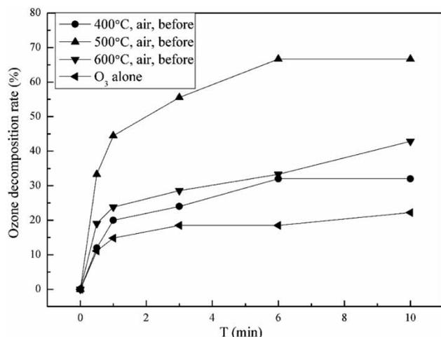
Figure 6 | Ozone decomposition rate with different catalysts.
