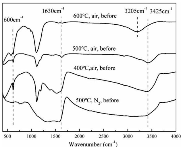
**Figure 4** | FT-IR spectra of different catalysts before experiments.
