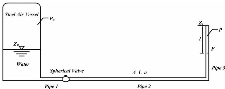
Figure 1 | Schematic diagram of pipeline system layout.
