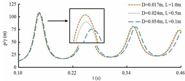
**Figure 6** | Air pocket pressure versus time with different diameter and length of air pocket.
