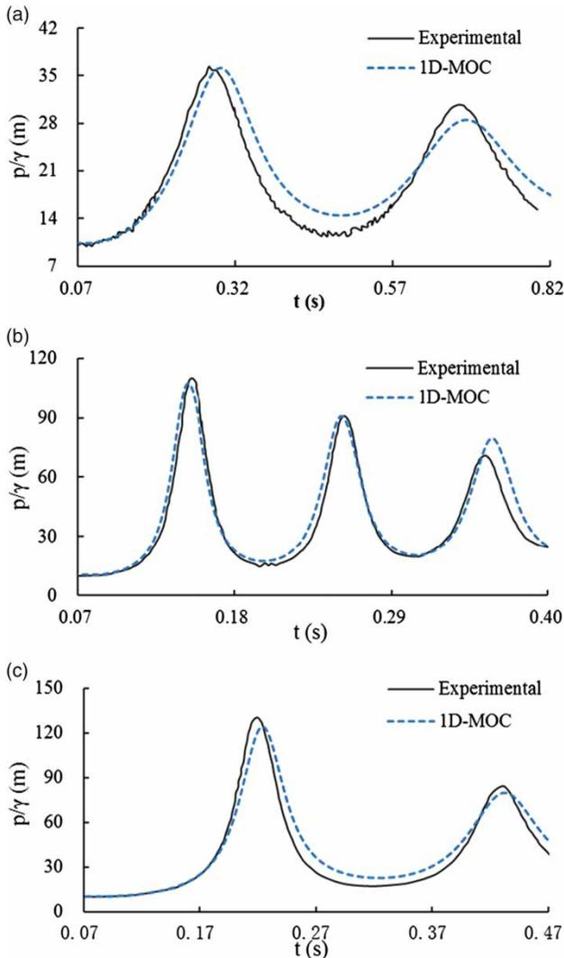
**Figure 2** | Air pocket pressure comparison under three conditions: (a) condition a ( $h_0 = 1$ ,  $L_{air0}/D = 9.3$ ); (b) condition b ( $h_0 = 1$ ,  $L_{air0}/D = 1.9$ ); (c) condition c ( $h_0 = 3$ ,  $L_{air0}/D = 9.3$ ).
