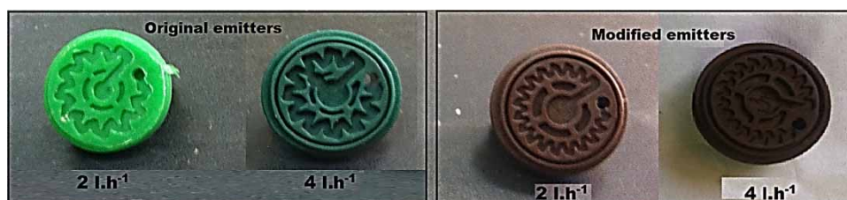
Figure 1 | Comparison between water path map for the standard and modified emitter.
