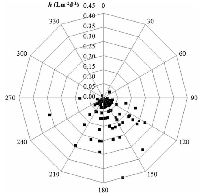
**Figure 9** | Daily dew yields versus wind direction averaged during the night (21:00 to 6:00); north:  $0^\circ$ ; east:  $90^\circ$ ; south:  $180^\circ$ ; west:  $270^\circ$ .
