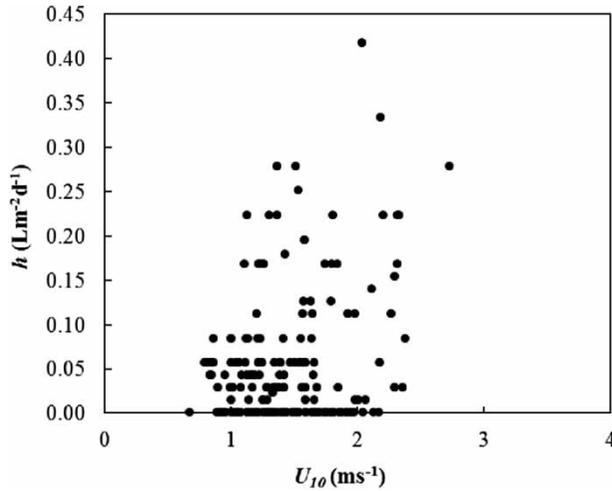
**Figure 8** | Daily dew yields versus wind speed at 10 m agl averaged during the night (21:00 to 06:00). Outliers ( $U_{10} > 3.5 \text{ m s}^{-1}$ ) were not plotted.
