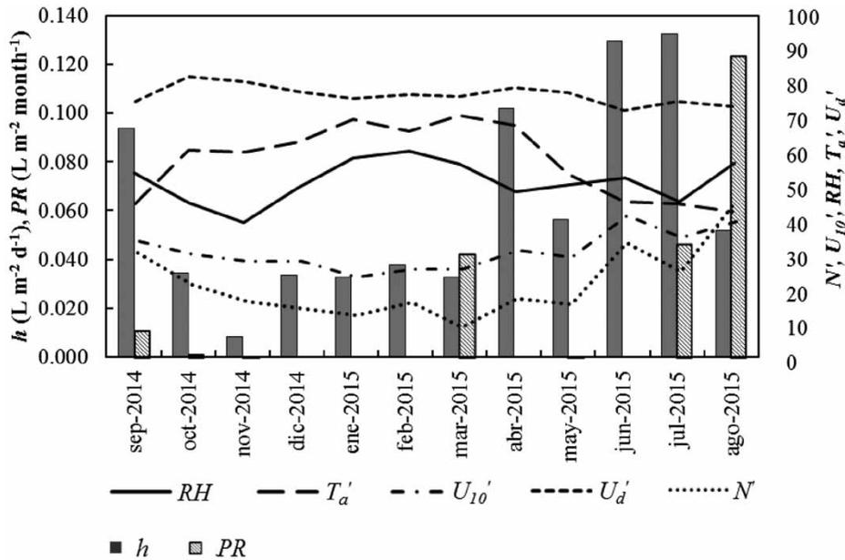
**Figure 4** | Monthly daily average dew yields, monthly rainfall, and meteorological data (from 21:00 to 06:00). Meteorological data were normalized as follows:  $N' = 10 N$ ,  $U_{10}' = 20 U_{10}$ ,  $T_a' = 4 T_a$ ,  $U_d' = U_d/2$ . Meteorological data for which daily dew yield was missing were omitted.
