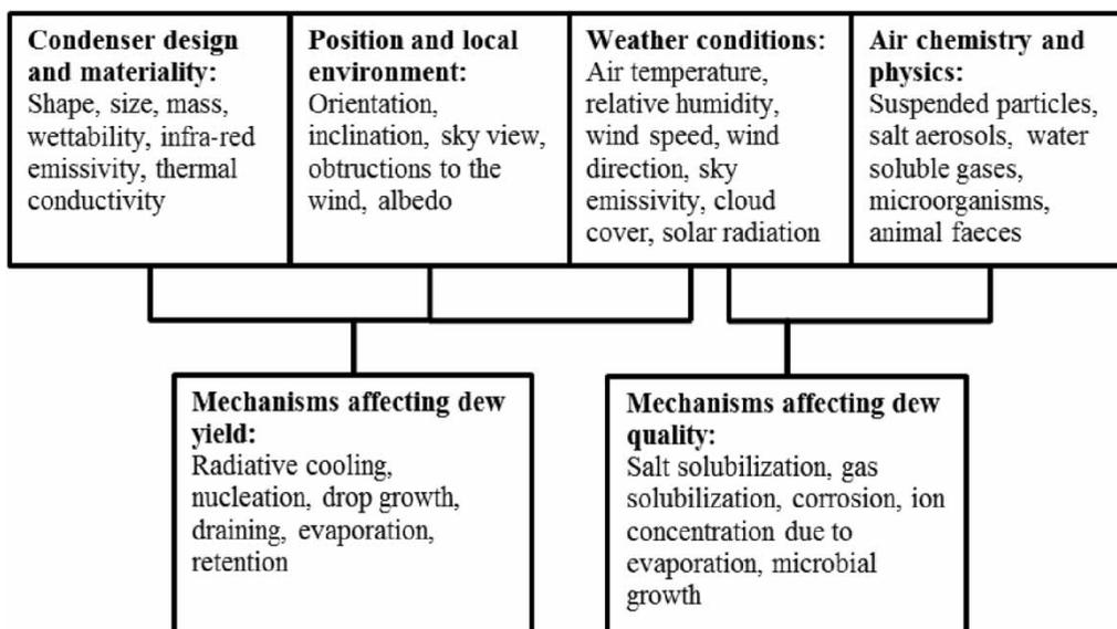
**Figure 1** | Diagram of the factors affecting dew yields and water quality of a passive dew condenser.
