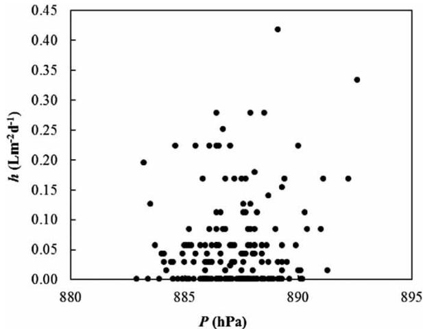
**Figure 11** | Daily dew yields versus atmospheric pressure averaged during the night (21:00–6:00). Pressure sensor: Vaisala/PTB110. Location: Observatorio Cruz del Sur, CEAZA.
