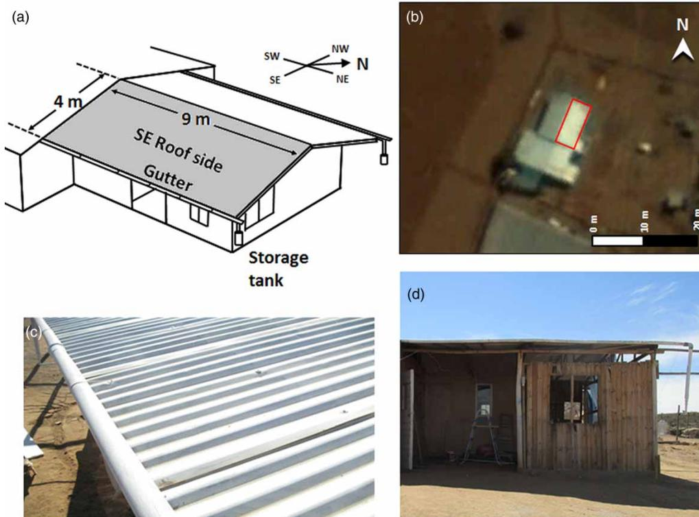
**Figure 3** | (a) Schematic sketch of the household with a modified rooftop for dew collection; (b) satellite image of the study site (Google Earth 2018); (c) photograph of the roof; and (d) photograph of the south-eastern façade.
