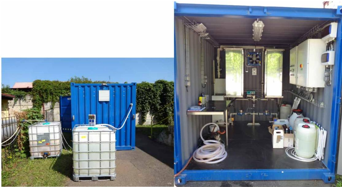
**Figure 2** | The appearance of the pilot scale unit, operated on an industrial site, in a container: left, outside view; right, interior of container with two visible reactors.
