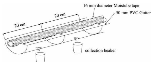
Figure 1 | Setup for the determination of the coefficient of variation.
