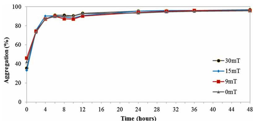
Figure 1 | Aggregation of sludge samples with and without magnetic field exposure.
