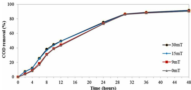
Figure 4 | Profile of COD removal performance throughout the operational period with and without magnetic field exposure.
