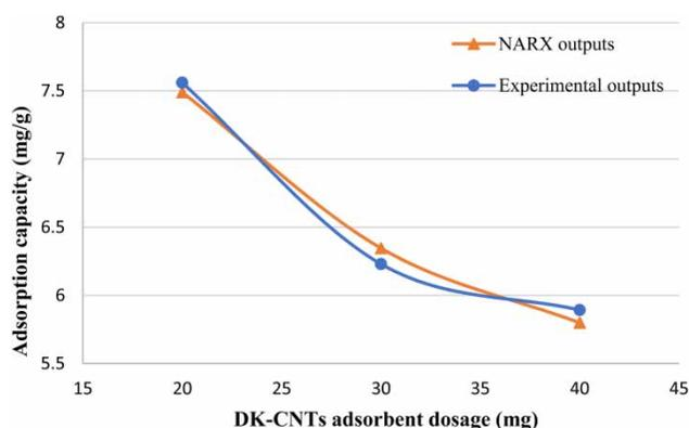
Figure 6 | Experimental and NARX outputs as a function of adsorbent dosage.
