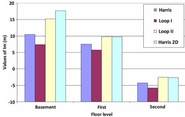
**Figure 4** | Variations of the minimum surplus head ( $l_m$ ) at the different floors and configurations.
