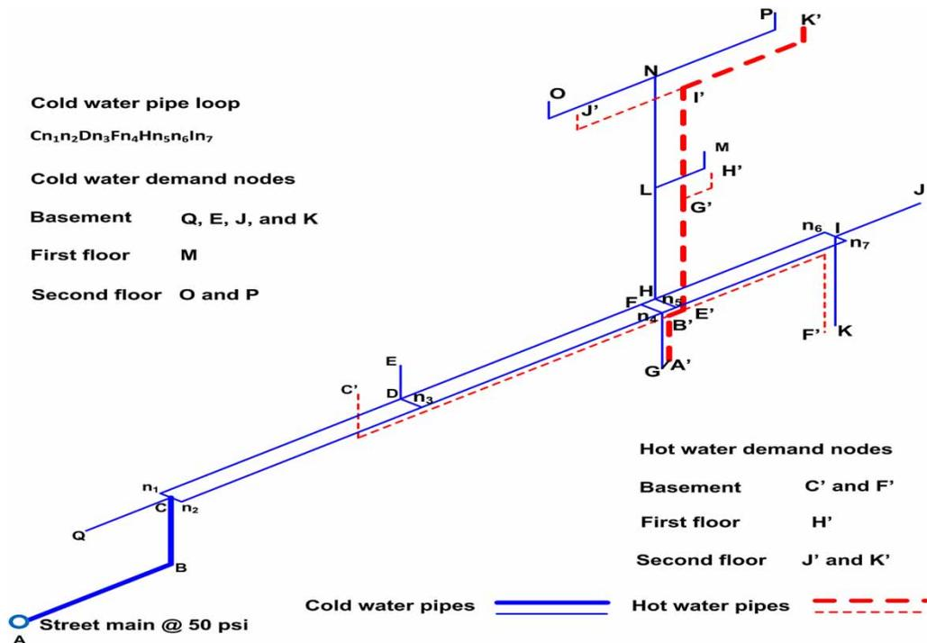
Figure 2 | Looped I configuration layout.
