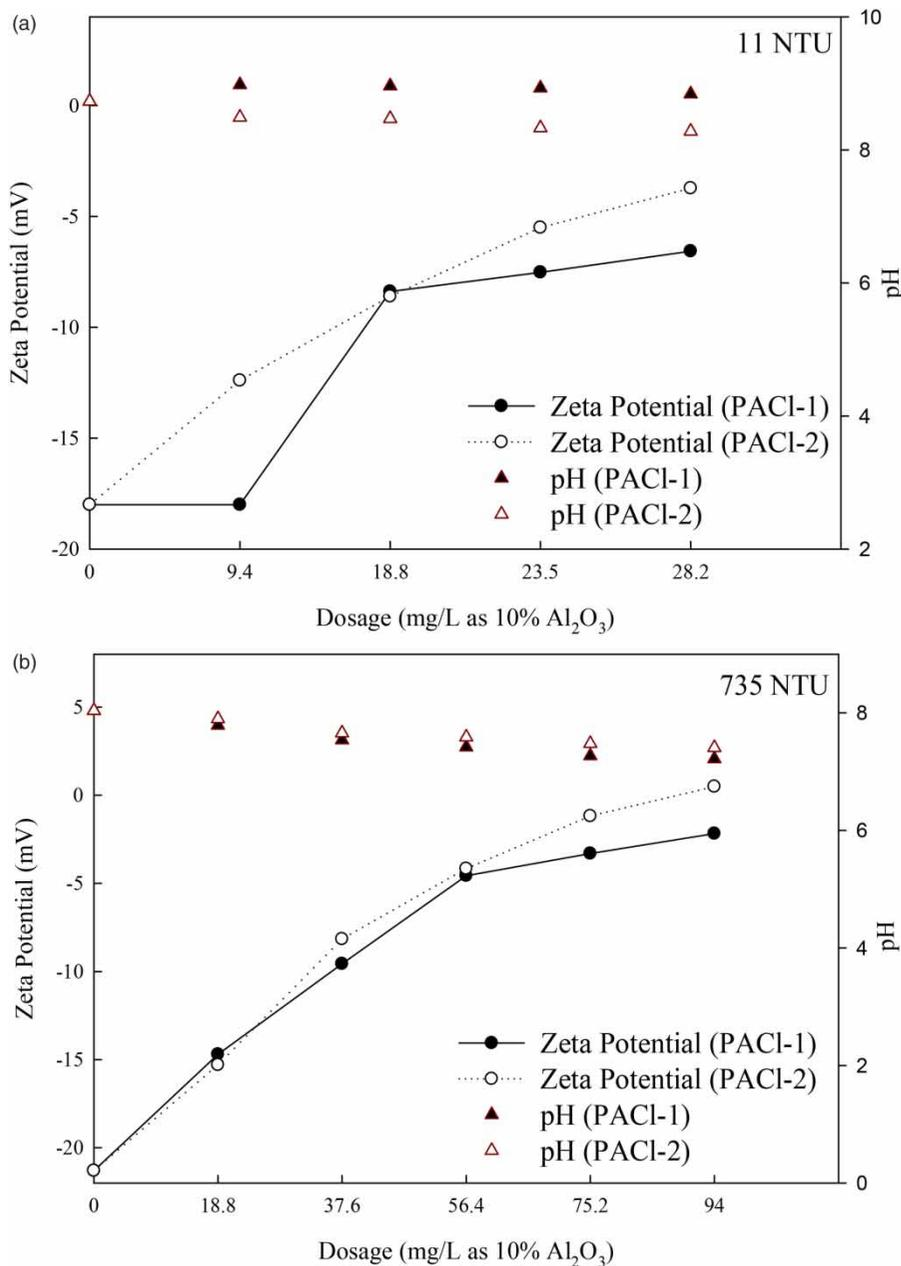
**Figure 3** | Comparison in zeta potential changes with corresponding pH by coagulation with either PACI-1 or PACI-2 at various dosages for low and high turbid water: (a) 11 NTU and (b) 735 NTU.
