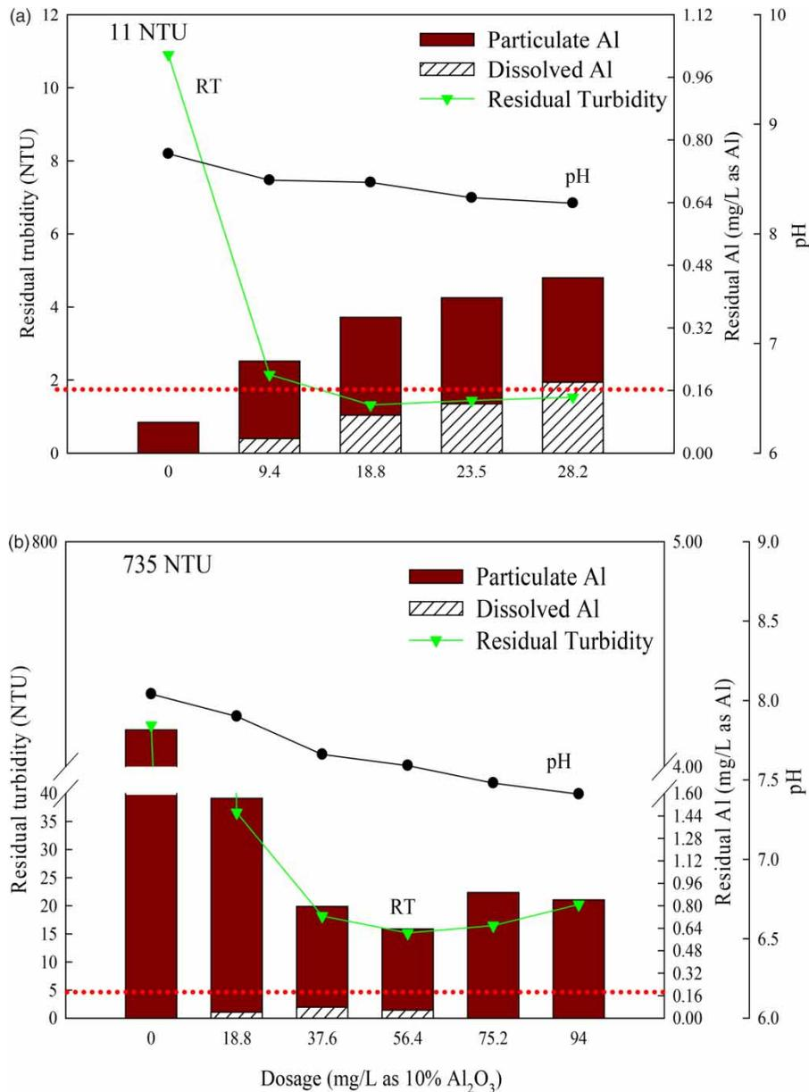
**Figure 2** | Variations of residual turbidity and Al of supernatant and corresponding pH by coagulation with PACI-2 at various dosages for low and high turbid water: (a) 11 NTU and (b) 735 NTU.
