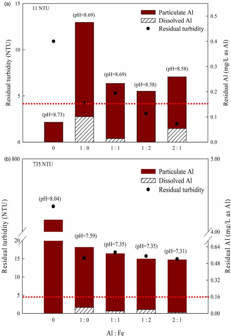
**Figure 5** | The relationship between pH, residual turbidity, and Al of supernatant at various ratios of mixed PACI-2 and  $\text{FeCl}_3$  coagulant: (a) 11 NTU and (b) 735 NTU.
