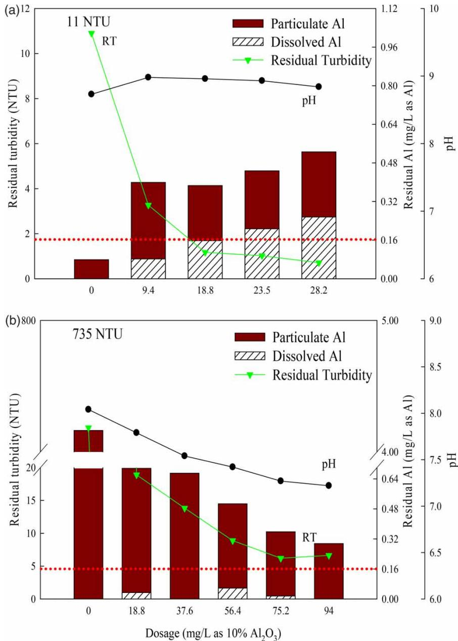
**Figure 1** | Variations of residual turbidity and Al of supernatant and corresponding pH by coagulation with PACI-1 at various dosages for low and high turbid water: (a) 11 NTU and (b) 735 NTU.
