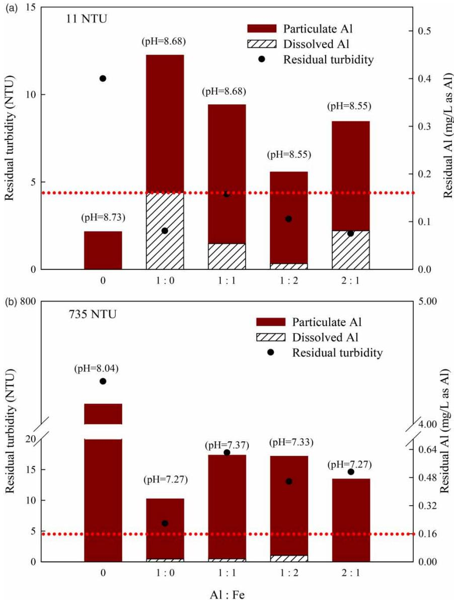
**Figure 4** | The relationship between pH, residual turbidity, and Al of supernatant at various ratios of mixed PACl-1 and FeCl<sub>3</sub> coagulant for low and high turbidity water: (a) 11 NTU and (b) 735 NTU.
