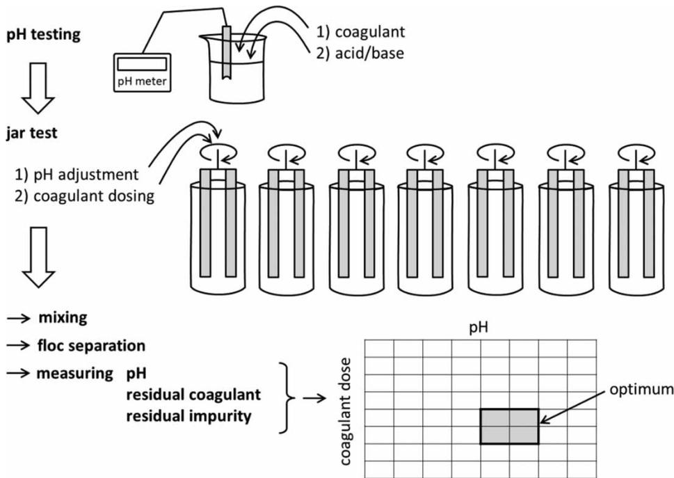
Figure 1 | Recommended procedure of coagulant dosage and pH optimization.
