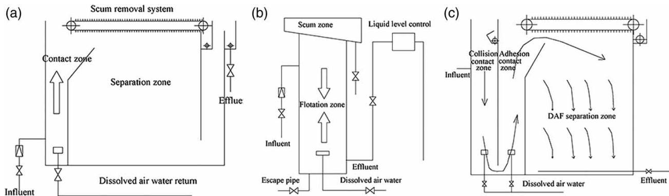
**Figure 1** | Sketch of the cocurrent DAF process (a), countercurrent DAF process (b), and CCDAF process (c).
