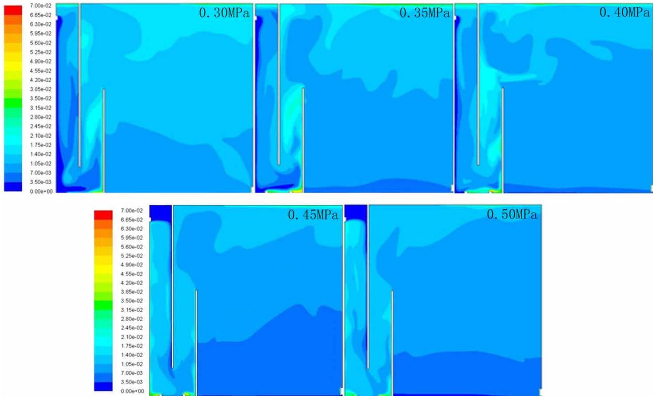
**Figure 7** | Contour of bubble fraction in CCDAF tank under different pressures of dissolved gas (0.30–0.50 MPa).
