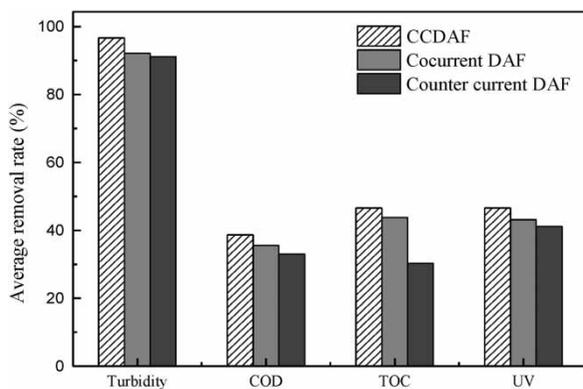
**Figure 9** | Comparison of removal effects of different processes under optimal conditions.
