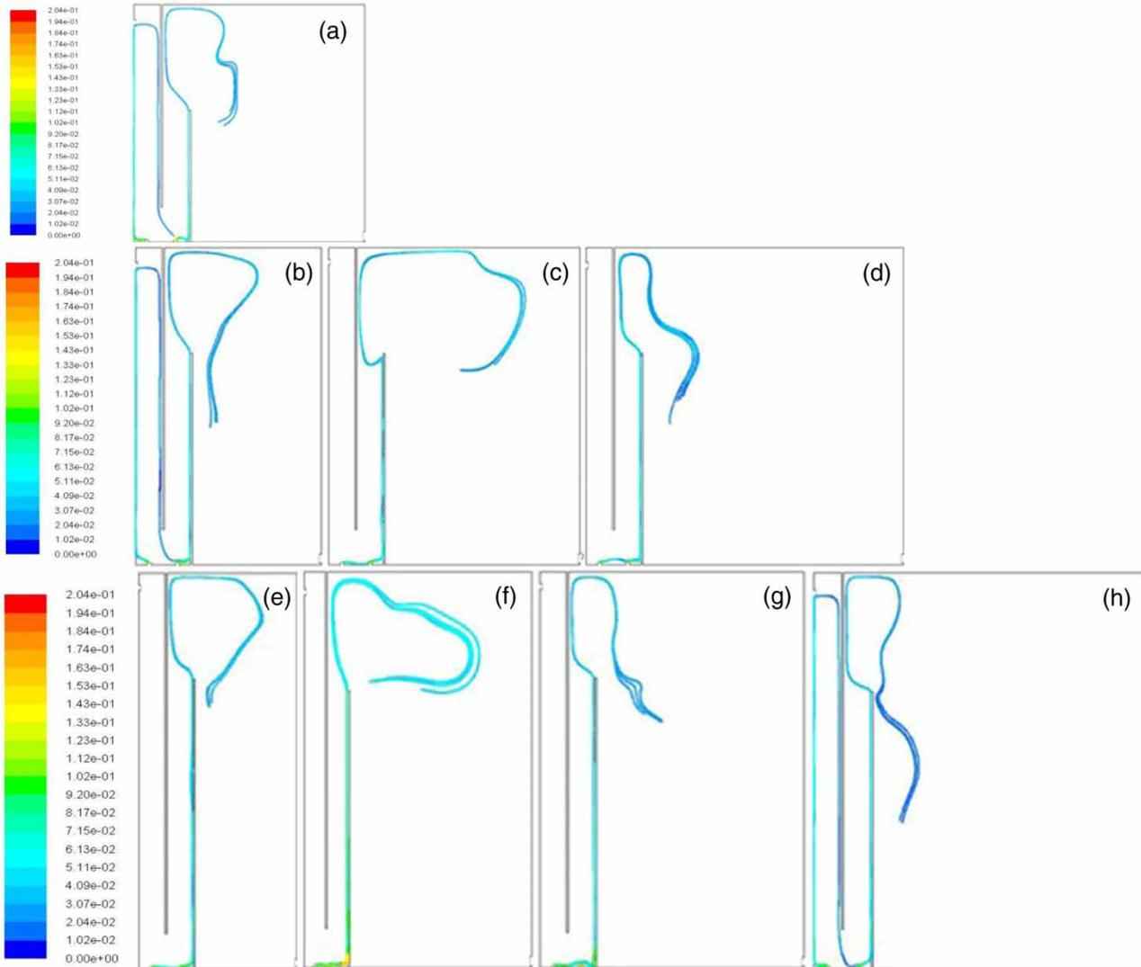
**Figure 5** | Pathlines of gas-phase velocity of eight models in the CCDAF tank (a)–(h).
