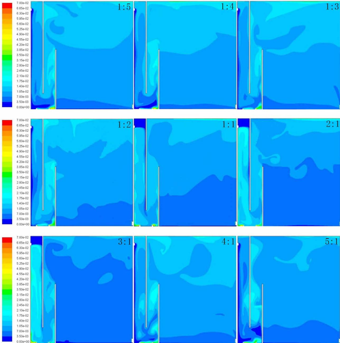
**Figure 8** | Contour of bubble fraction of different distribution ratios of reflux gas-dissolved water at the inlet (1:5–5:1).
