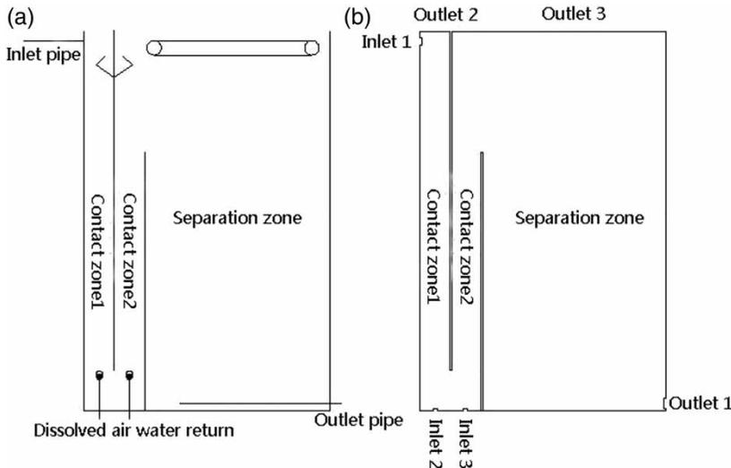
**Figure 2** | Sketch of the air flotation tank (a) and model (b).
