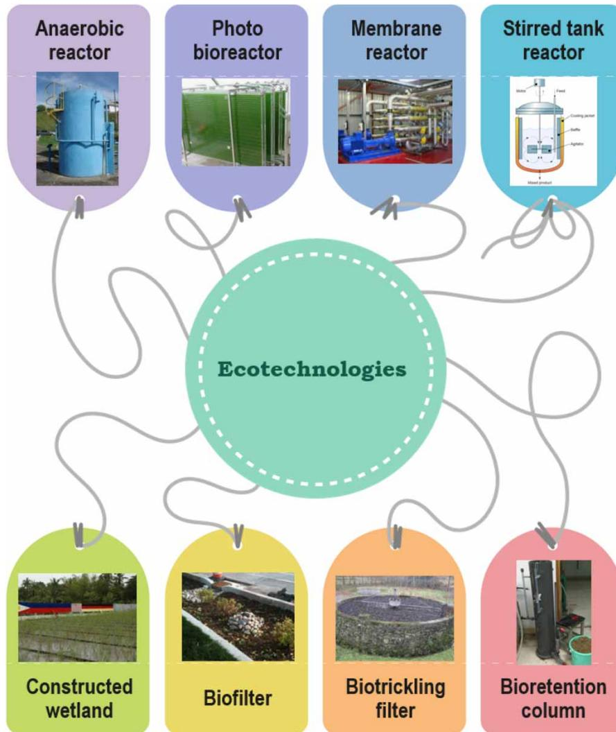
**Figure 1** | Representative ecotechnologies used for water, wastewater treatment and resource recovery. Most of these technologies use naturally available resources (e.g. micro-organisms or packing material or plant species) for treating the pollutant.
