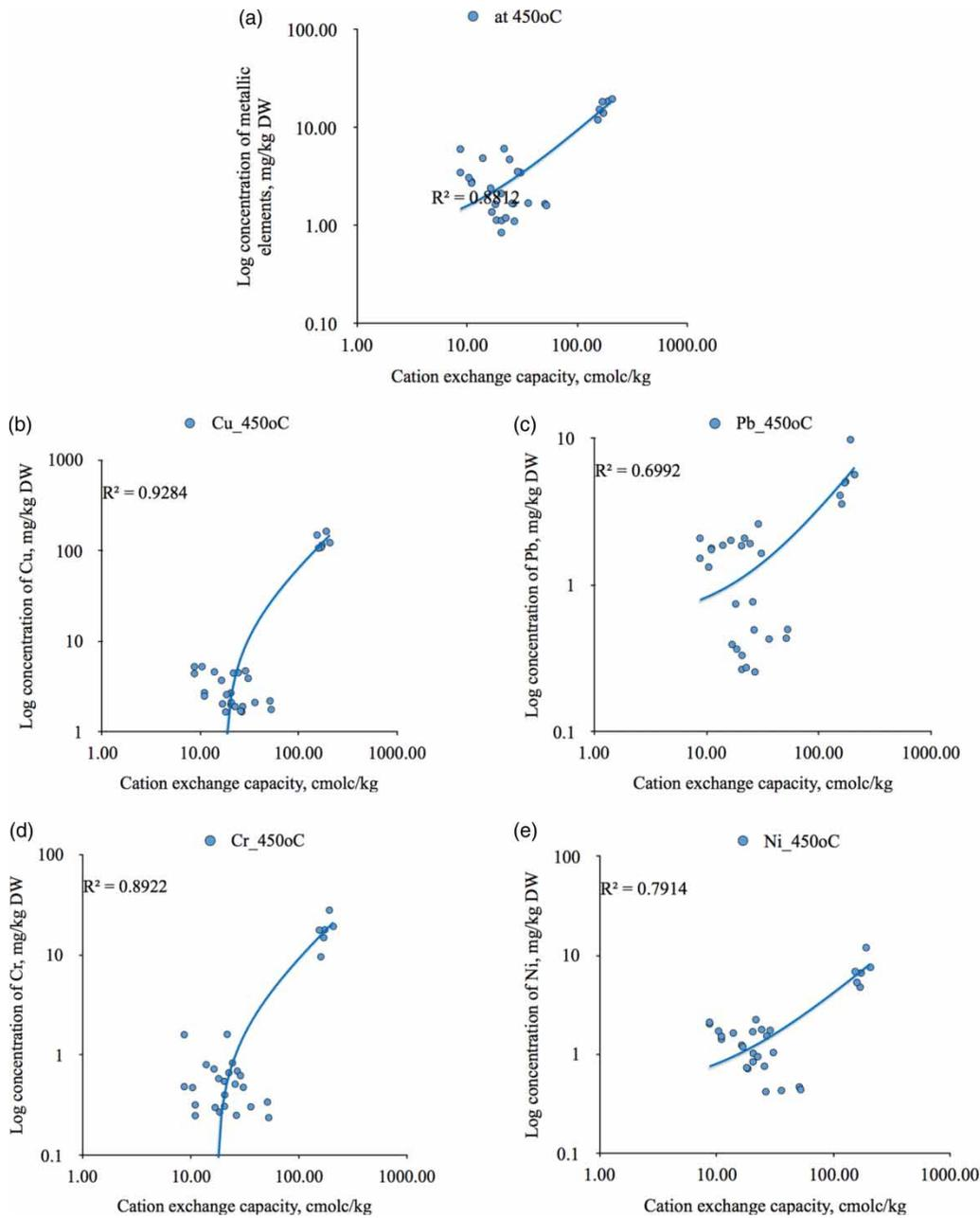
**Figure 5** | Logarithmic relationship between cation exchange capacity and chemical element concentration in biochar: (a) for all chemical elements at 450 °C; (b) for Cu at 450 °C; (c) for Pb at 450 °C; (d) for Cr at 450 °C; (e) for Ni at 450 °C.
