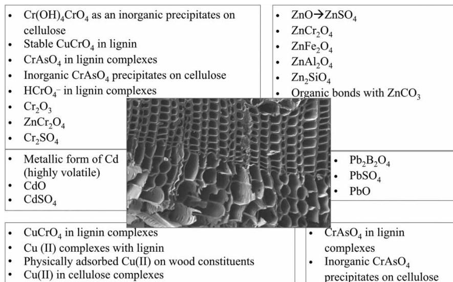
**Figure 3** | List of metallic element phases which are found in biochar produced at a temperature of about 750 °C. The image in the figure presents the structural view (magnification 300×) of biochar.
