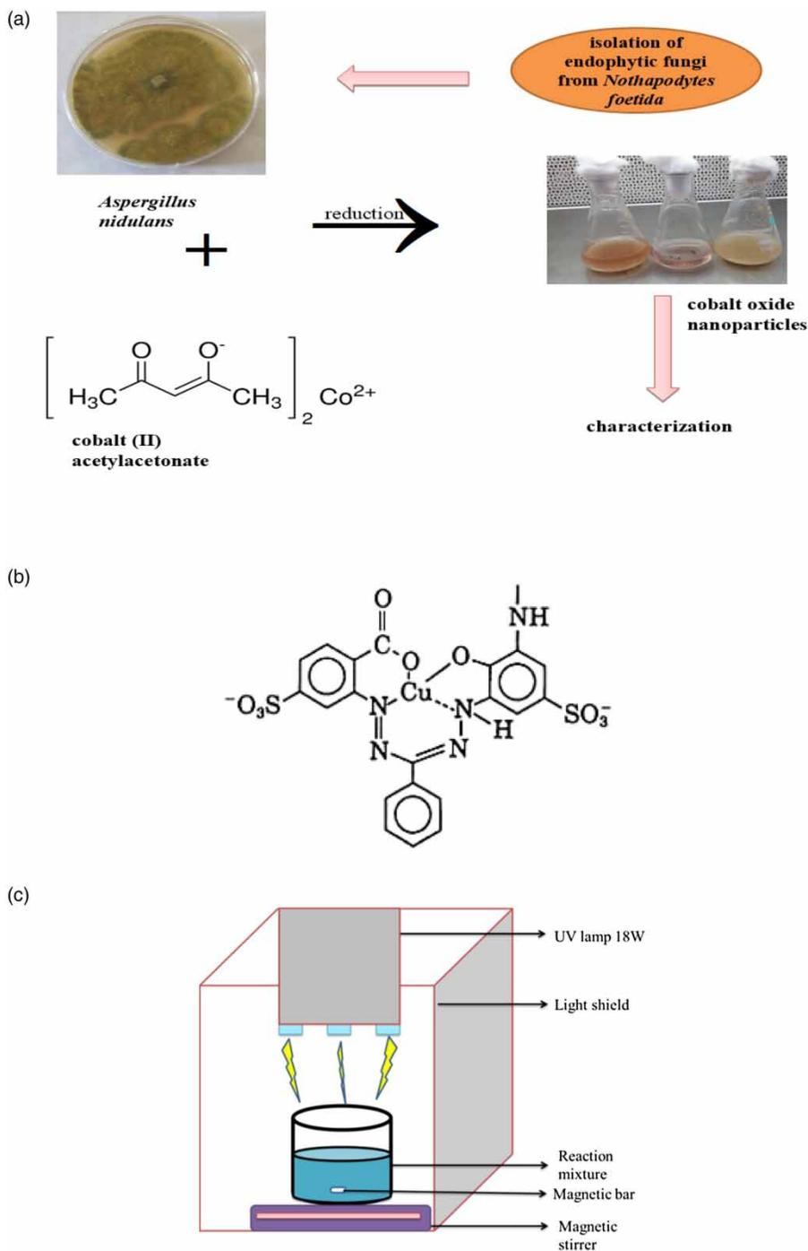
**Figure 1** | (a) Synthesis of cobalt oxide nanoparticles (Vijayanandan & Balakrishnan 2018), (b) structure of RB220 dye (Bodurođlu et al. 2014), and (c) experimental set-up for RB220 degradation.
