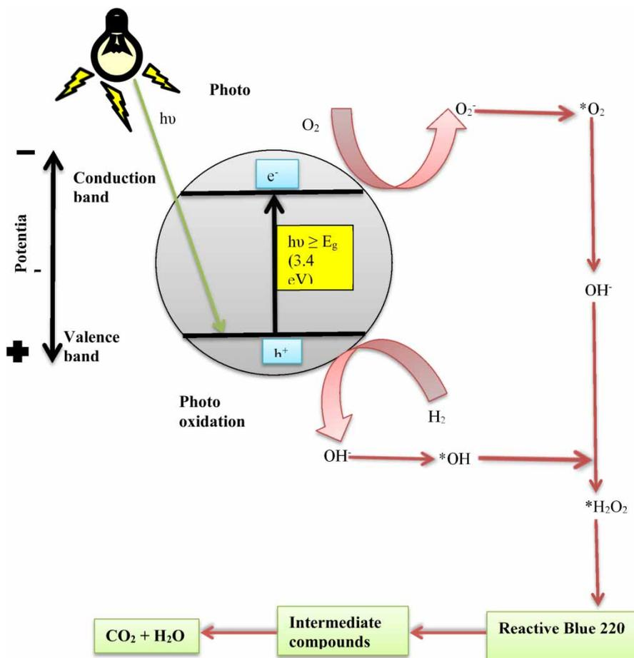
Figure 4 | Mechanism of RB220 degradation by hydroxyl radicals.
