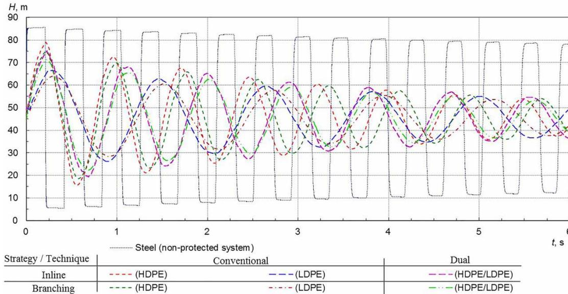
Figure 3 | Downstream pressure head signals, for the non- and protected system cases using the inline or branching strategy based on the dual or conventional technique.
