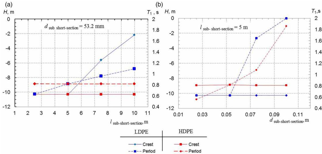
**Figure 7** | Sensitivity of the first pressure head crest and the period of the 1st cycle of pressure wave oscillations to the plastic sub-short-sections: (a) lengths (for  $d_{\text{sub-short-section}} = 53.2$  mm) and (b) diameters (for  $l_{\text{sub-short-section}} = 5$  m), for the (LDPE-HDPE)-branching set-up-based controlled system.
