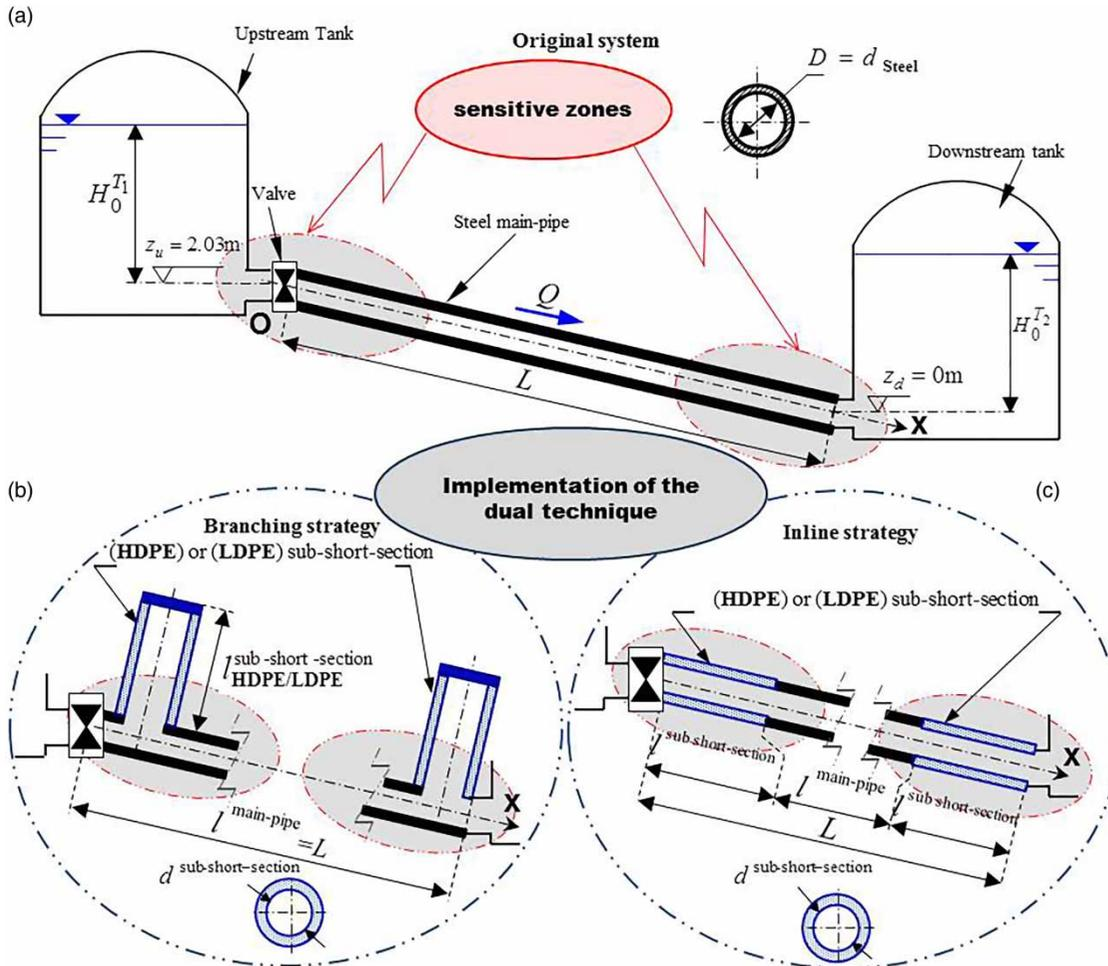
**Figure 5** | Sketch of the hydraulic system for the negative-surge control test case: (a) the original system and the controlled system using the dual technique-based (b) branching and (c) inline strategy.
