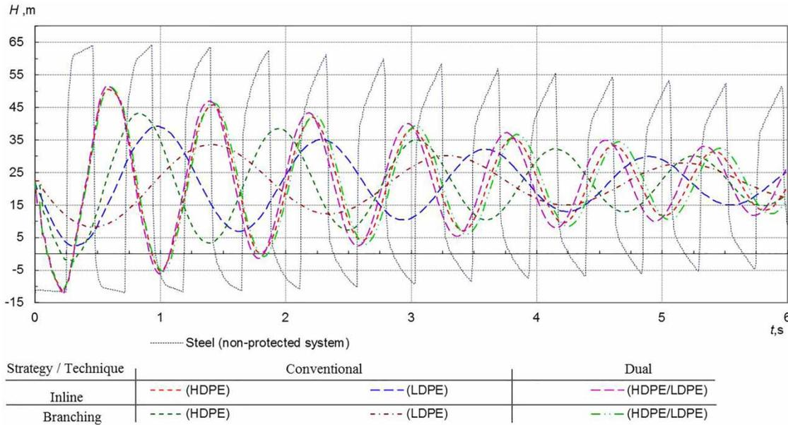
Figure 6 | Upstream pressure head signals for the non-protected and protected systems based on the dual and conventional techniques.
