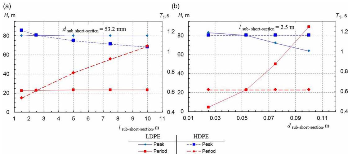
**Figure 4** | Sensitivity of the first pressure head peak and the period of the 1st cycle of pressure wave oscillations to the plastic sub-short-sections: (a) lengths (for  $d_{\text{sub-short-section}} = 53.2$  mm) and (b) diameters (for  $l_{\text{sub-short-section}} = 2.5$  m), for the (LDPE-HDPE)-branching set-up-based controlled system.
