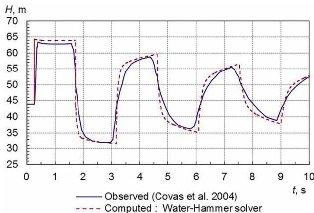
Figure 1 | Comparison between experimental and numerical pressure head traces.
