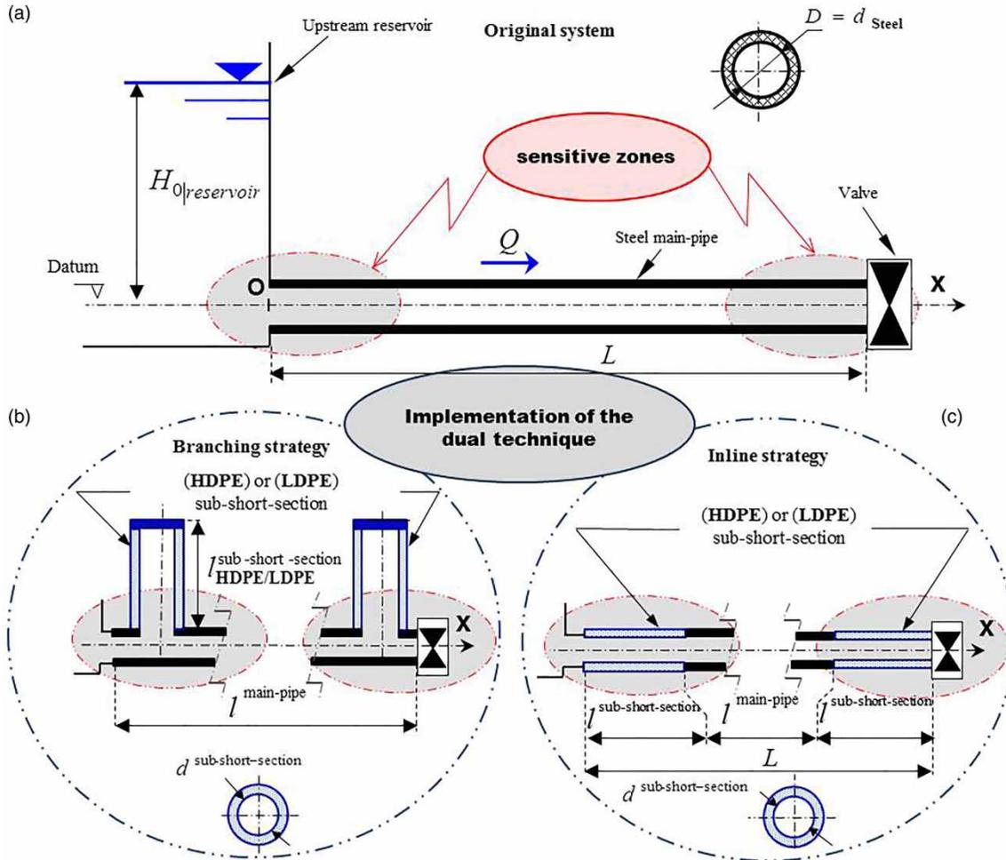
**Figure 2** | Sketch of the hydraulic system for the positive-surge control test case: (a) the original system and the controlled system using the dual technique-based (b) branching or (c) inline strategy.
