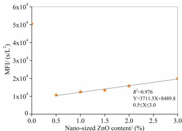
**Figure 7** | Effect of ZnO content on the MFI values of the prepared membranes.
