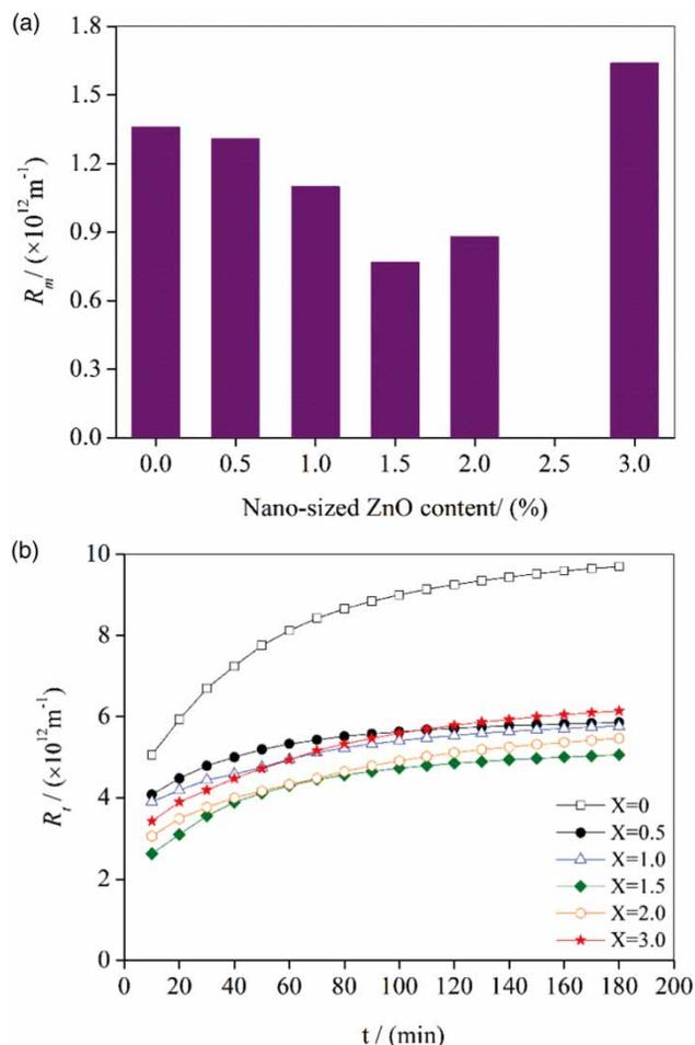
**Figure 6** | Effect of nano-ZnO content on filtration resistance: (a) membrane resistance and (b) total filtration resistance of BSA.
