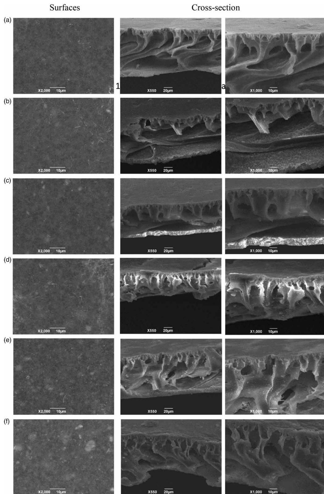
**Figure 1** | SEM images of surfaces and cross sections for the PVDF/ZnO-X membranes: (a) X = 0; (b) X = 0.5; (c) X = 1.0; (d) X = 1.5; (e) X = 2.0; (f) X = 3.0.
