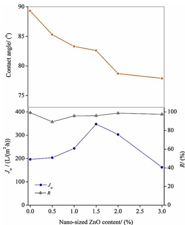
**Figure 5** | Pure water fluxes and BSA rejection of the membranes.
