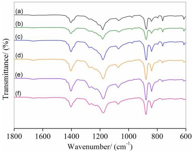
**Figure 2** | FTIR spectra for the PVDF/ZnO-X membranes: (a) X = 0; (b) X = 0.5; (c) X = 1.0; (d) X = 1.5; (e) X = 2.0; (f) X = 3.0.
