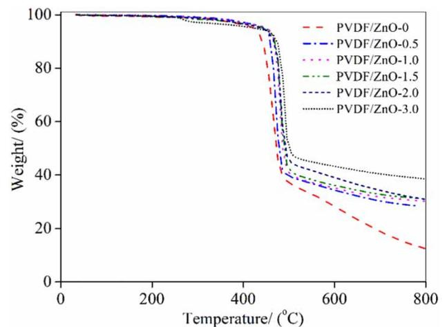
**Figure 4** | TGA for neat and ZnO-embedded PVDF membrane.
