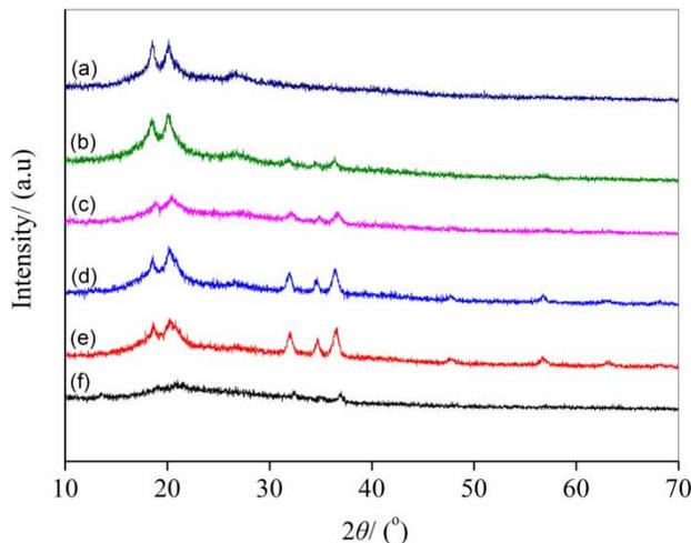
**Figure 3** | XRD patterns of PVDF/ZnO-X membranes: (a) X = 0; (b) X = 0.5; (c) X = 1.0; (d) X = 1.5; (e) X = 2.0; (f) X = 3.0.
