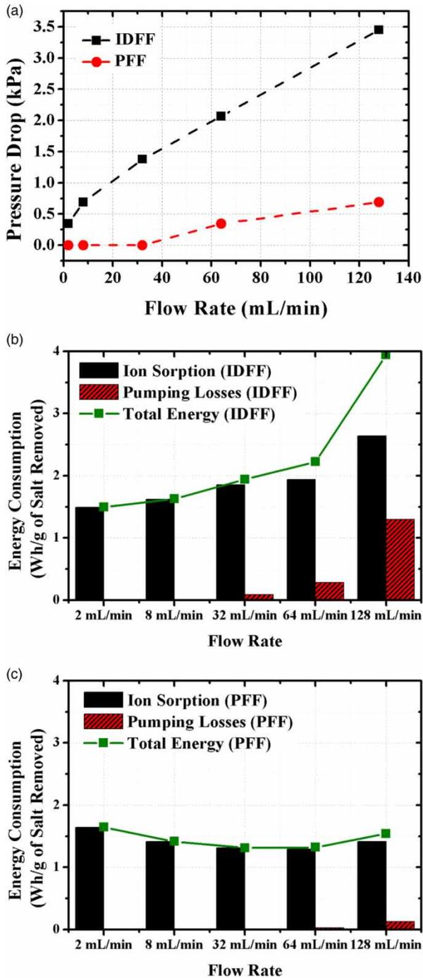
**Figure 6** | (a) Pressure drop vs flow rate plots for IDFF and PFF, energy consumption vs flow rate plots for (b) IDFF, and (c) PFF.
