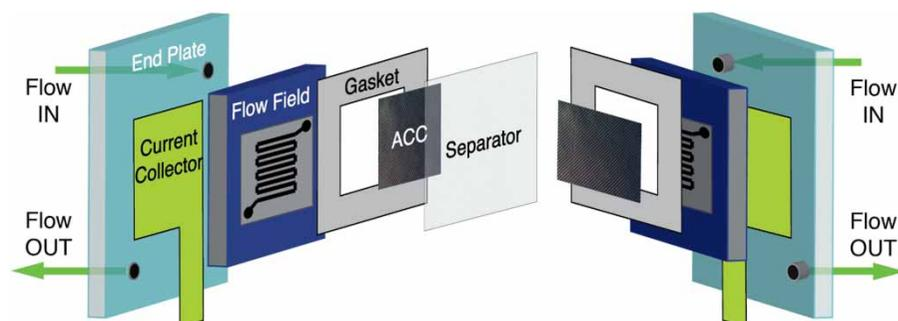
Figure 1 | CDI cell schematic.
