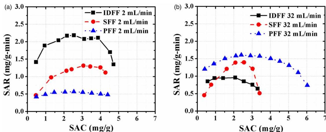
**Figure 5** | *In situ* SAR vs SAC plot of different flow field designs at (a) 2 and (b) 32 mL/min flow rates.
