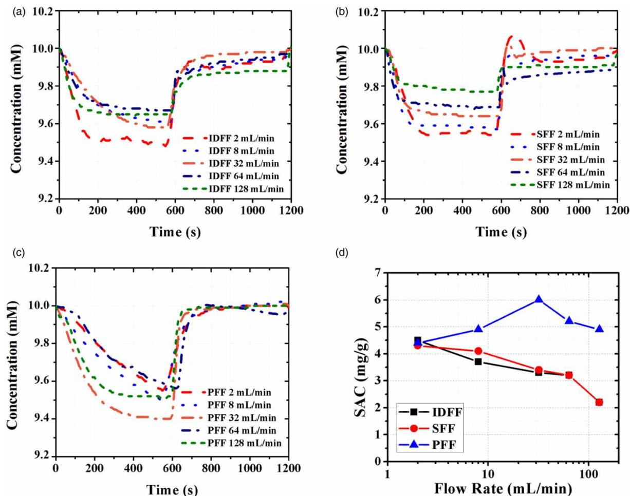
Figure 3 | Concentration vs time plots for (a) IDFF, (b) SFF, (c) PFF, and (d) SAC vs flow rate plot.
