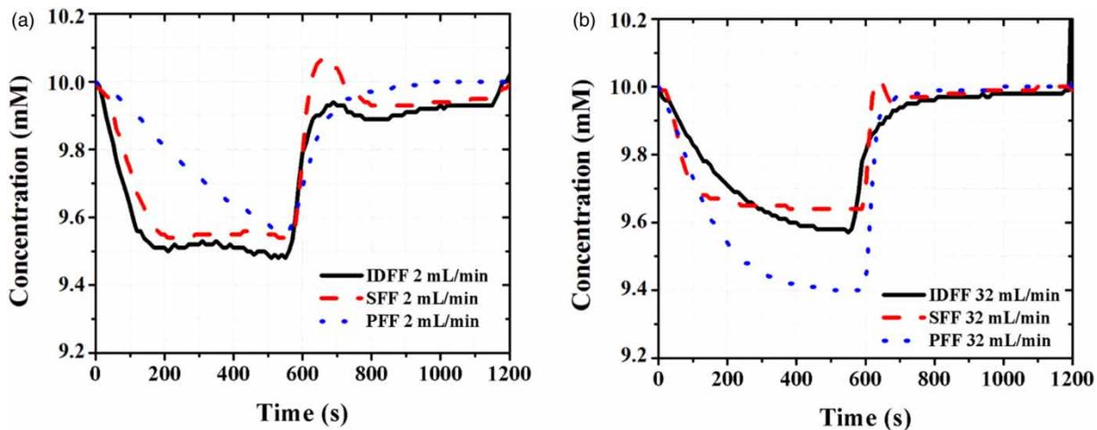
Figure 4 | Concentration vs time plots for all FF designs at (a) 2 and (b) 32 mL/min flow rates.
