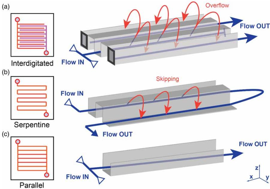
**Figure 2** | Schematic of (a) IDFF, (b) SFF, and (c) PFF designs.
