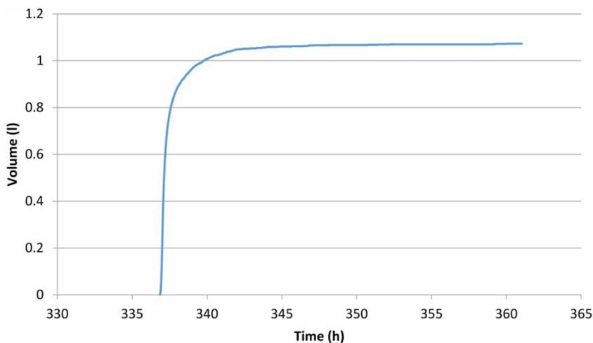
**Figure 9** | Discharged volume achieved 7 hr after the start of outflow production in week 3, day 2 test.
