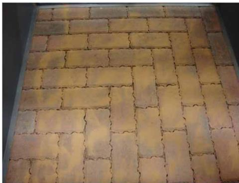
Figure 14 | Sediment load application at the beginning of week 4, day 2.
