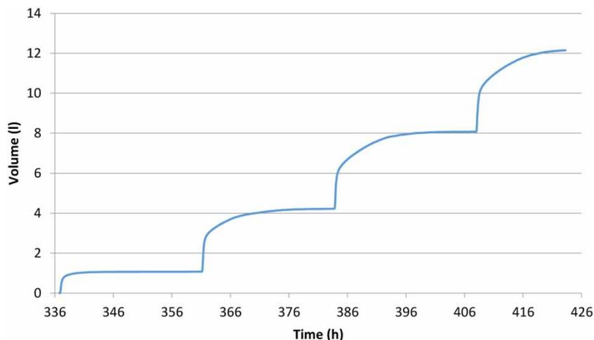
Figure 12 | Cumulative volume of water discharged from the pavement structure during week 3.
