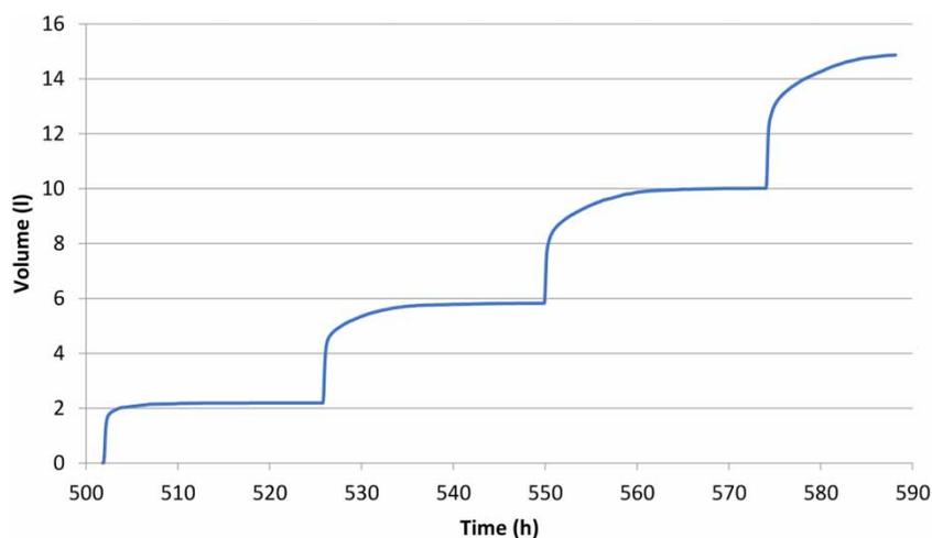
Figure 13 | Cumulative volume of water discharged from the pavement structure during week 4.
