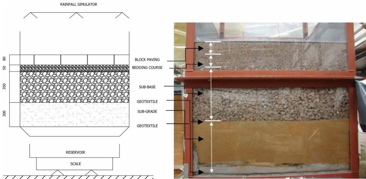
**Figure 2** | (Left) Schematic of the vertical cross section of the rig pavement illustrating the total vertical installation. Dimensions on the vertical axis are in mm. (Right) Picture of cross section of the pavement structure (Ioannidou & Arthur 2018).
