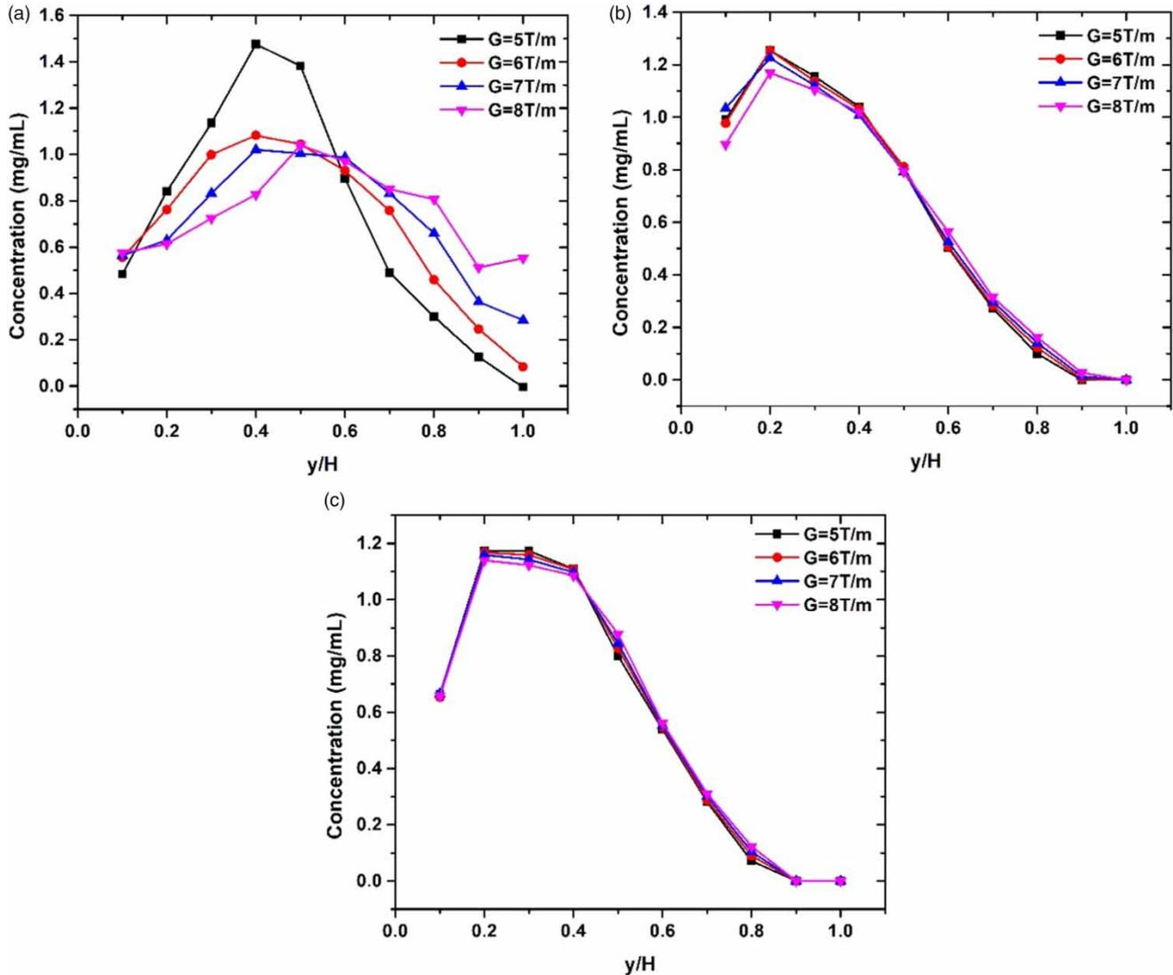
**Figure 4** | Particles' concentration for  $B_0 = 0.5\text{ T}$  and different magnetic gradients for (a)  $f = 5\text{ Hz}$ , (b)  $f = 10\text{ Hz}$ , (c)  $f = 15\text{ Hz}$ .
