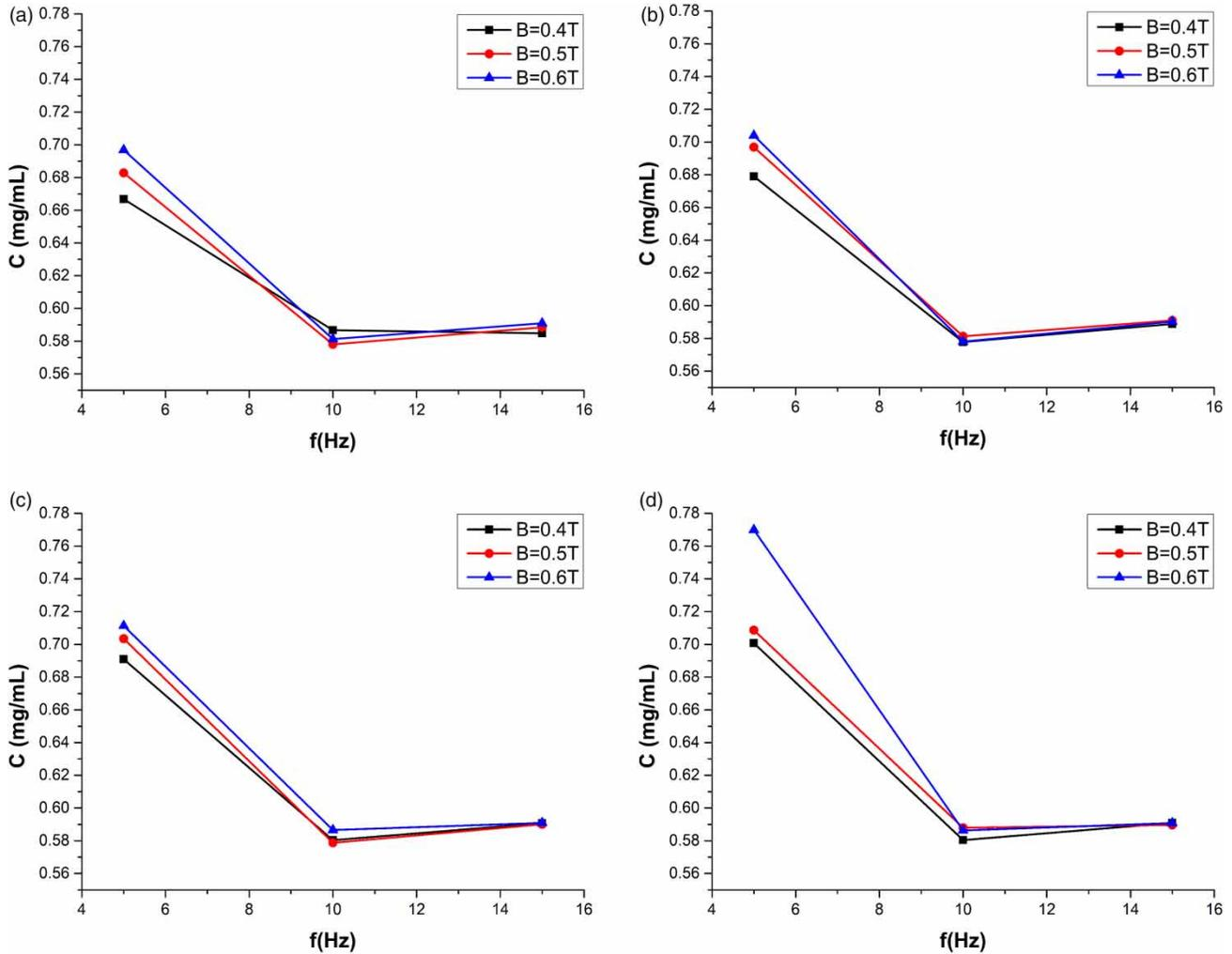
**Figure 6** | Mean concentration for different magnitudes of the magnetic field  $B_0$  for  $G$  equal to: (a) 5 T/m, (b) 6 T/m, (c) 7 T/m, and (d) 8 T/m.
