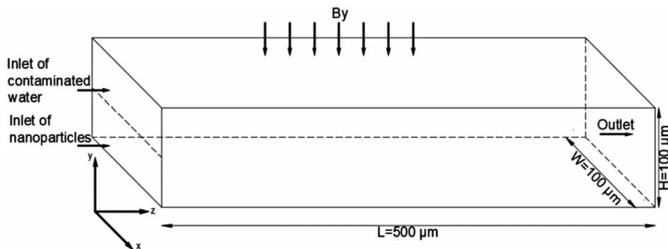
Figure 1 | Micromixer configuration and inflow/outflow conditions.
