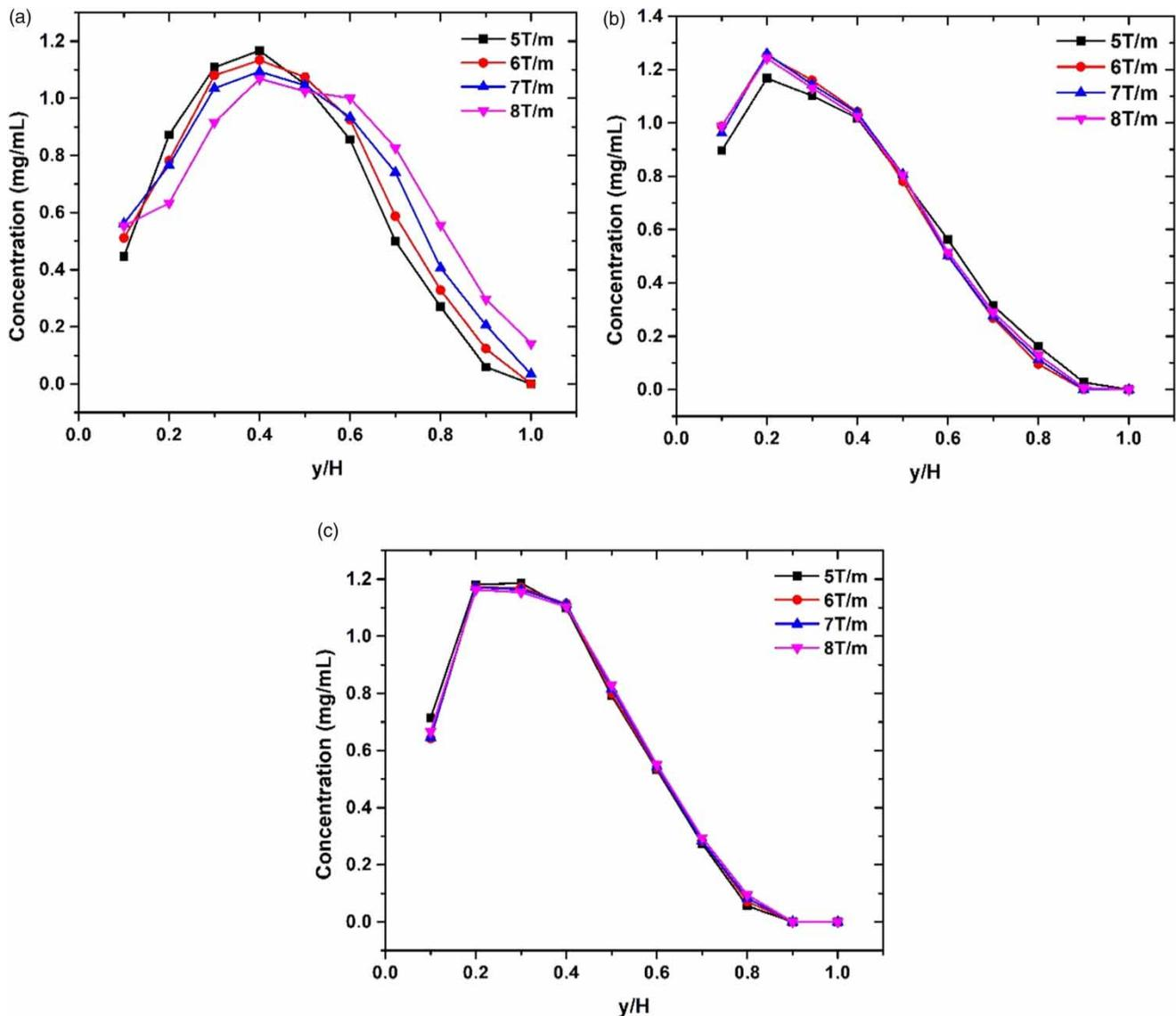
Figure 3 | Particles' concentration for  $B_0 = 0.4 \text{ T}$  and different magnetic gradients for (a)  $f = 5 \text{ Hz}$ , (b)  $f = 10 \text{ Hz}$ , (c)  $f = 15 \text{ Hz}$ .
