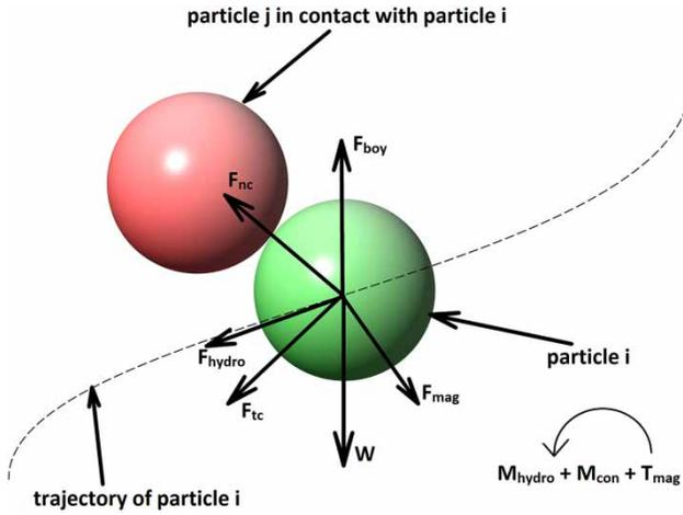
**Figure 2** | Schematic diagram of the forces acting on particles (Lampropoulos *et al.* 2015).
