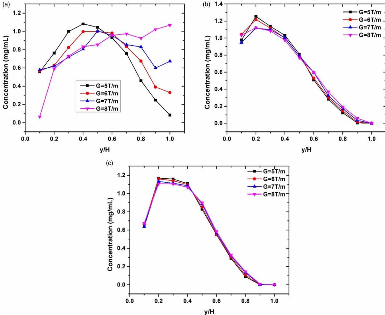
**Figure 5** | Particles' concentration for  $B_0 = 0.6$  T and different magnetic gradients for (a)  $f = 5$  Hz, (b)  $f = 10$  Hz, (c)  $f = 15$  Hz.
