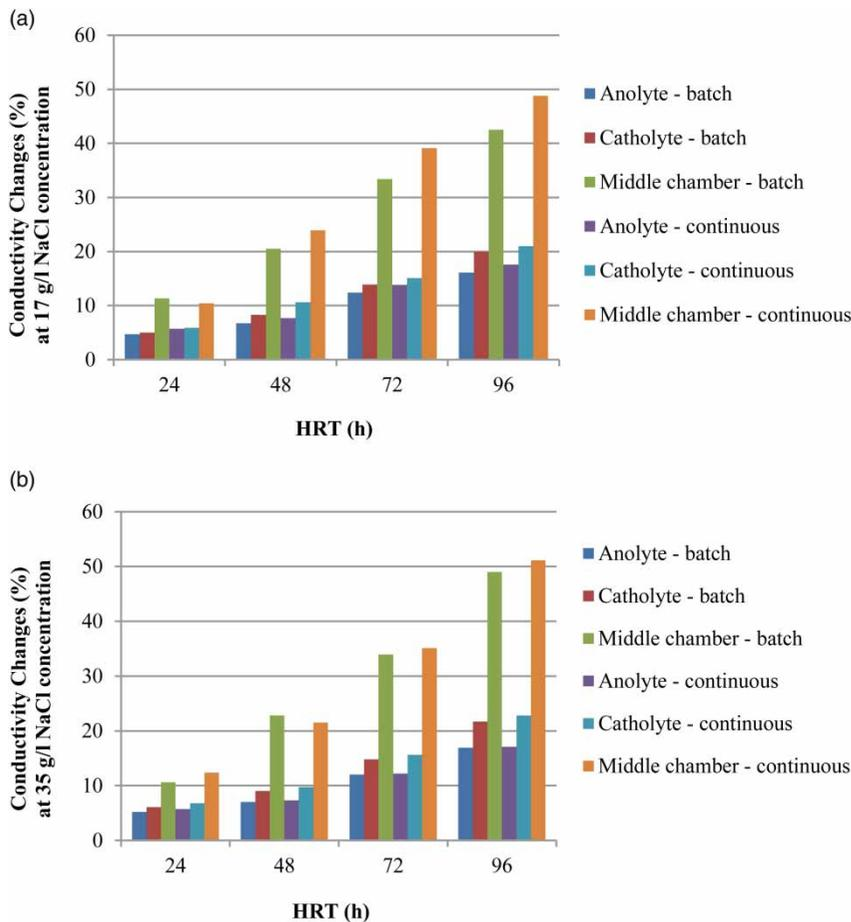
**Figure 4** | Changes of conductivity in electrode chambers during fed-batch mode and continuously fed mode: (a) performance at 17 g/L NaCl concentration; (b) performance at 35 g/L NaCl concentration.
