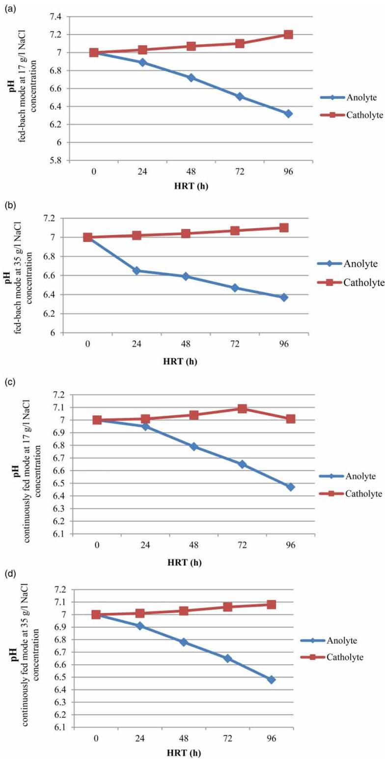
**Figure 5** | Changes of pH in electrode chambers: (a) fed-batch mode at 17 g/l NaCl concentration; (b) fed-batch mode at 35 g/l NaCl concentration; (c) continuously fed mode at 17 g/l NaCl concentration; (d) continuously fed mode at 35 g/l NaCl concentration.
