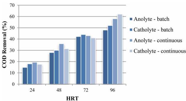
Figure 6 | COD removal efficiency (%) at 17 g/L NaCl concentration.
