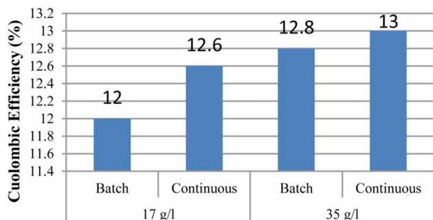
**Figure 8** | Coulombic efficiency (%) during batch and continuous mode at 17 and 35 g/L NaCl concentrations.
