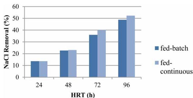
Figure 3 | Desalination performance at 35 g/L NaCl concentration.
