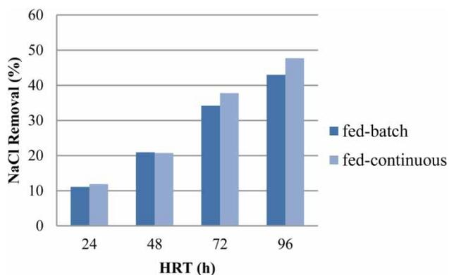
Figure 2 | Desalination performance at 17 g/L NaCl concentration.
