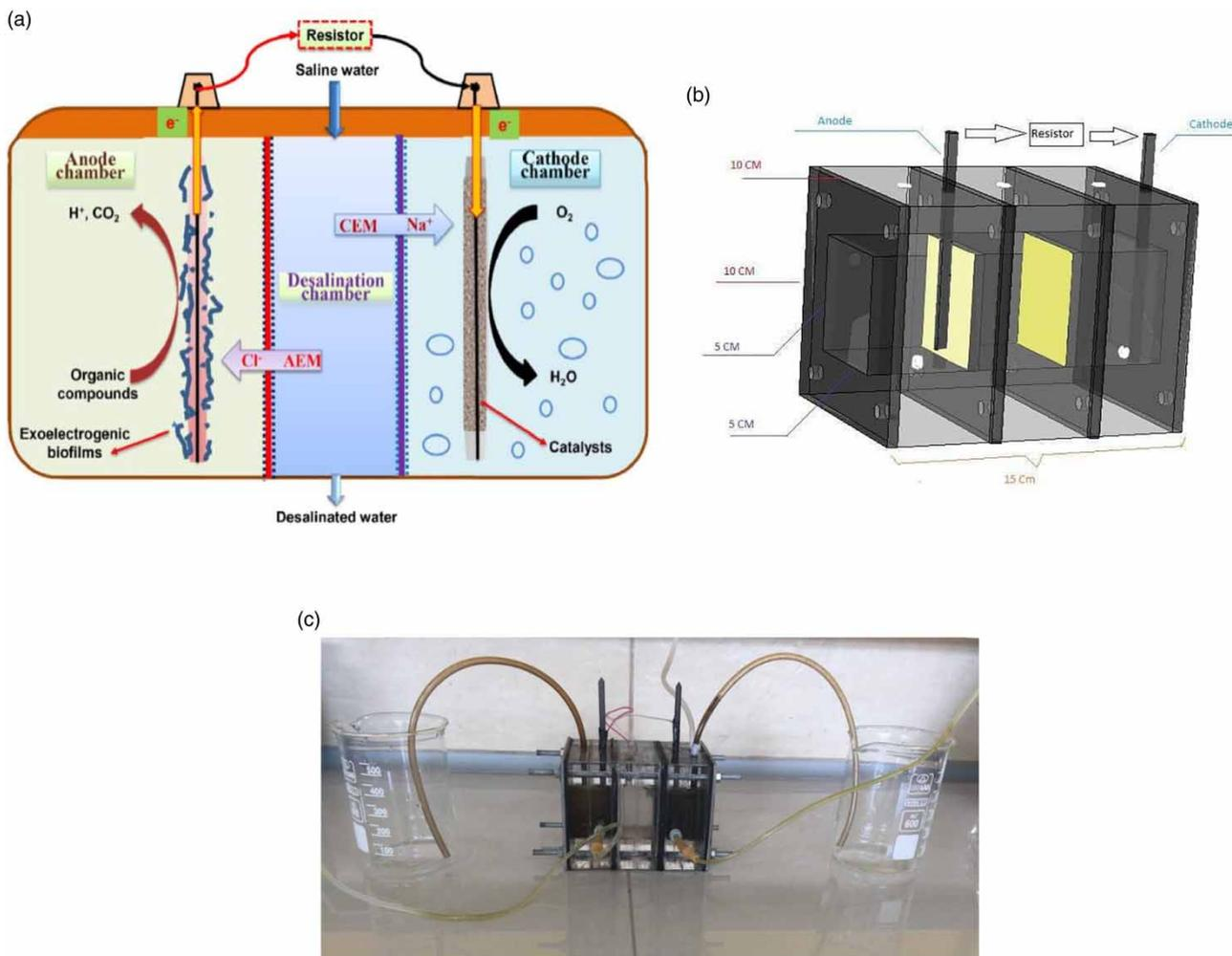
**Figure 1** | Three-chamber microbial desalination cell. AEM: Anion-exchange membrane, CEM: Cation-exchange membrane; (a) and (b) schematic, (c) photograph.
