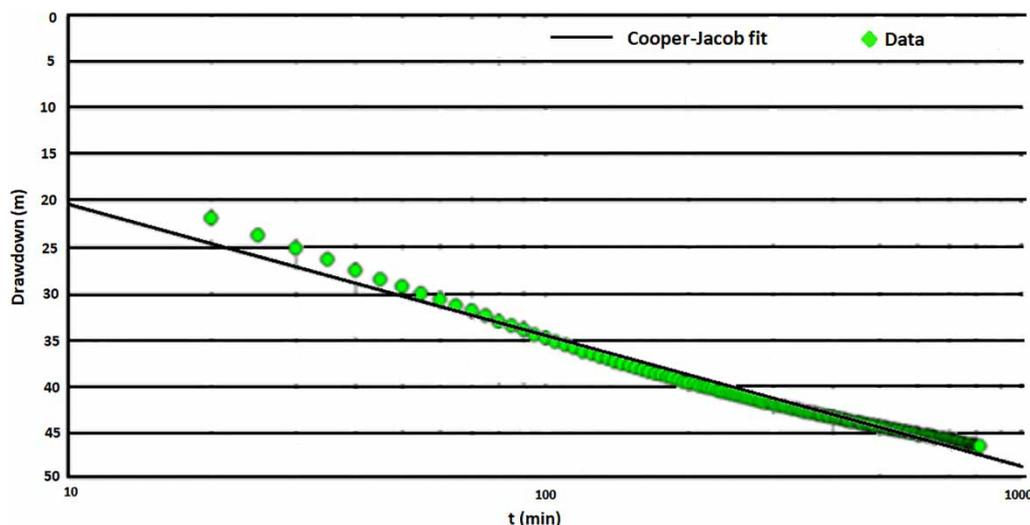
Figure 3 | Scatter plot from the AquiferTest showing the Cooper–Jacob model fit on drawdown data.
