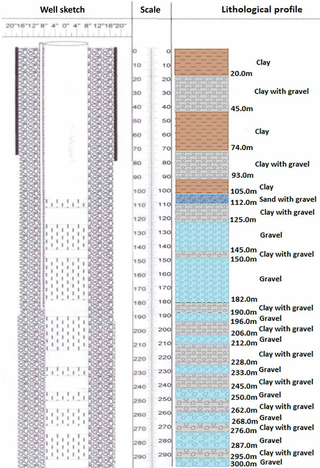
Figure 2 | Sketch of the investigated well and the soil layers that it encounters.
