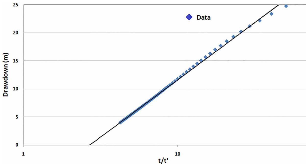
**Figure 8** | Application of the recovery method on the first set of 5-min residual drawdown data on 15 April 2018.
