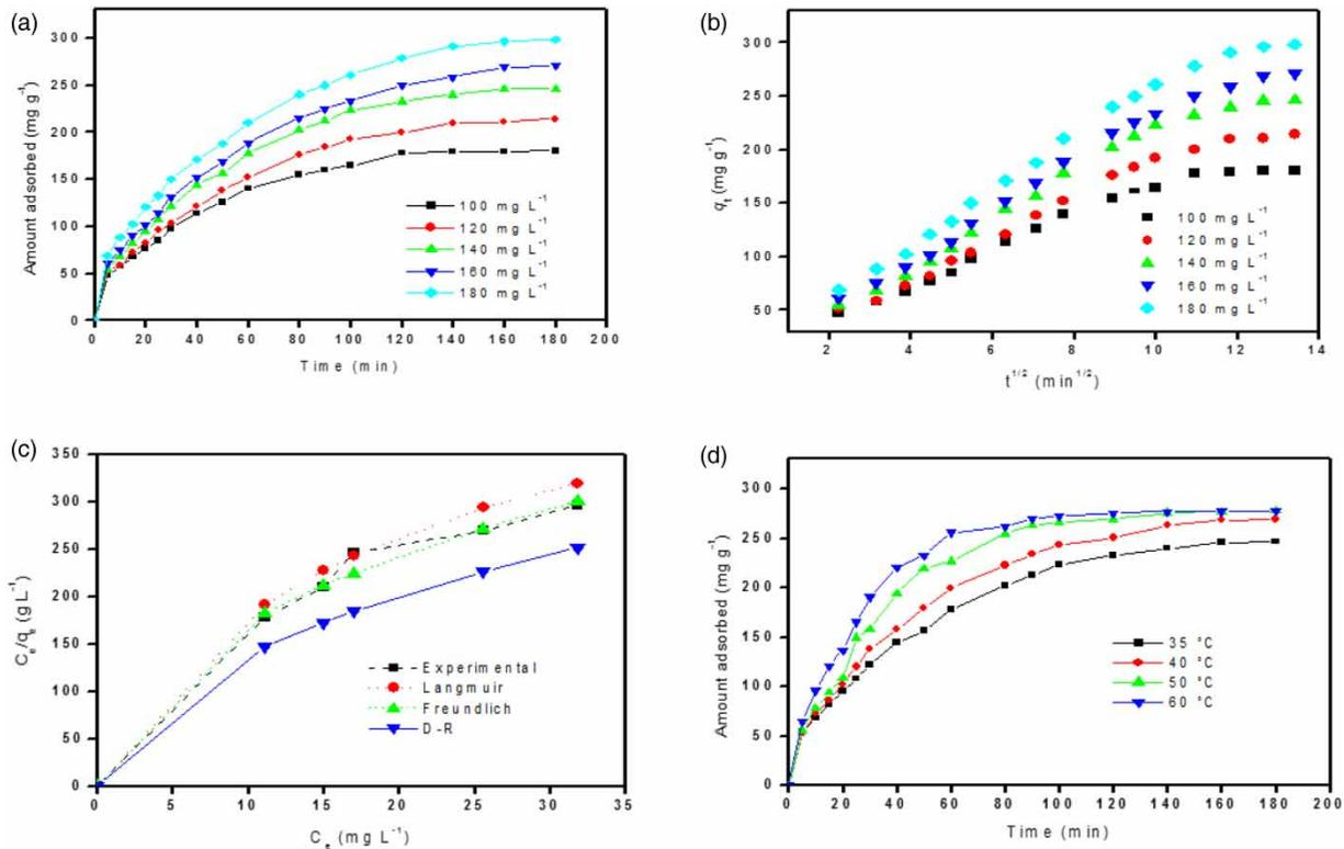
**Figure 5** | (a) Effect of agitation time and initial MB concentration on the amount of MB adsorbed by ZAJHC, (b) intraparticle diffusion plots for the adsorption of MB by ZAJHC, (c) comparison of Langmuir, Freundlich and D-R isotherms for the adsorption of MB by ZAJHC and (d) effect of temperature on the adsorption of MB by ZAJHC.
