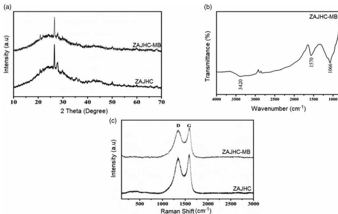
**Figure 2** | (a) X-ray diffraction patterns of ZAJHC and ZAJHC after adsorption of MB, (b) FTIR spectra of ZAJHC-MB and (c) Raman spectra of ZAJHC and ZAJHC after the adsorption of MB.
