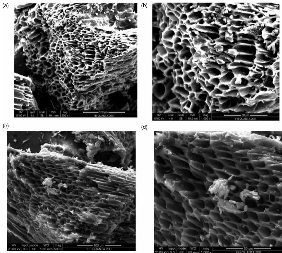
**Figure 3** | SEM images with different magnification images of (a) and (b) ZAJHC and (c) and (d) ZAJHC after the adsorption of MB.
