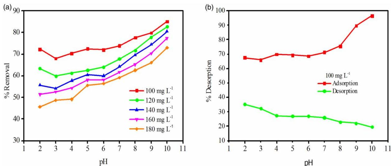
Figure 4 | Effect of pH on the (a) adsorption of MB by ZAJHC and (b) desorption of MB from ZAJHC.
