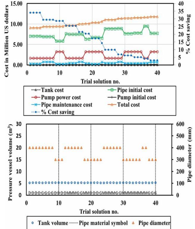
Figure 5 | Design output for the M-B&H pipeline.
