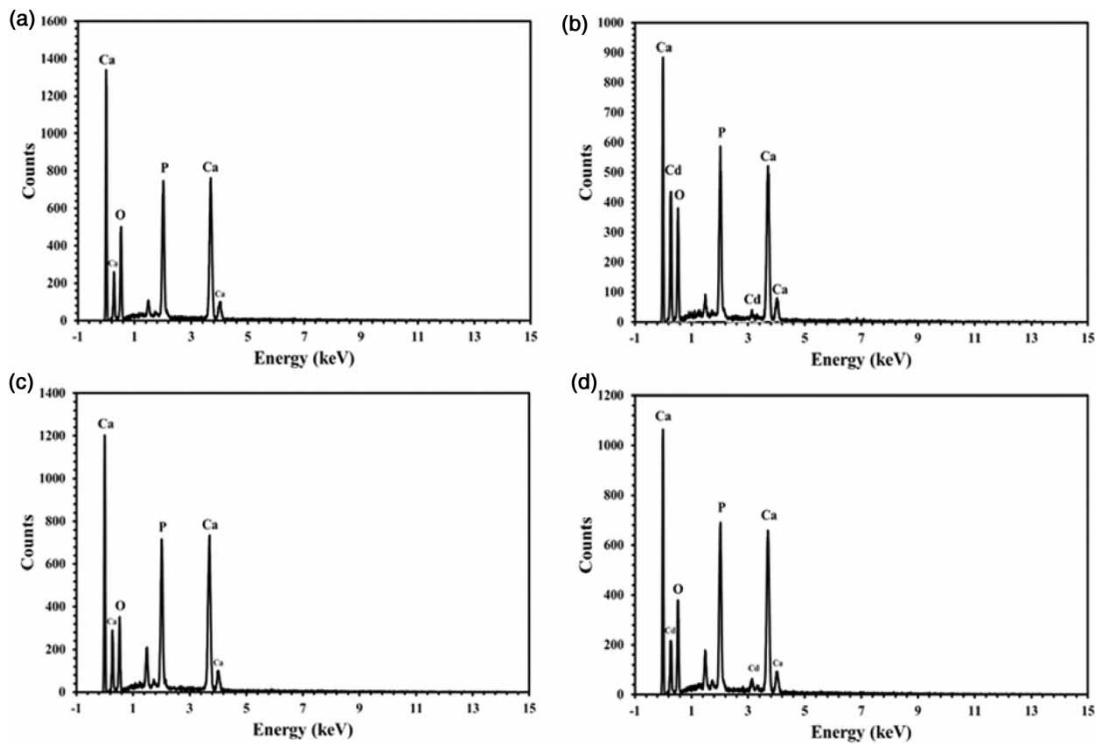
**Figure 12** | EDS graphs relative to HAP<sub>200</sub> (a), HAP<sub>200</sub>-Cd (b), HAP<sub>800</sub> (c), and HAP<sub>800</sub>-Cd (d).
