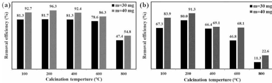
**Figure 3** | Evolution of Cd<sup>2+</sup> removal by adsorption onto HAP powders heated at various temperatures (a) at pH = 5.2 (b) at pH = 7 (Conditions: [Cd<sup>2+</sup>]<sub>0</sub> = 10 mg L<sup>-1</sup>, V = 100 mL, m = 30 and 40 mg, t = 120 min).
