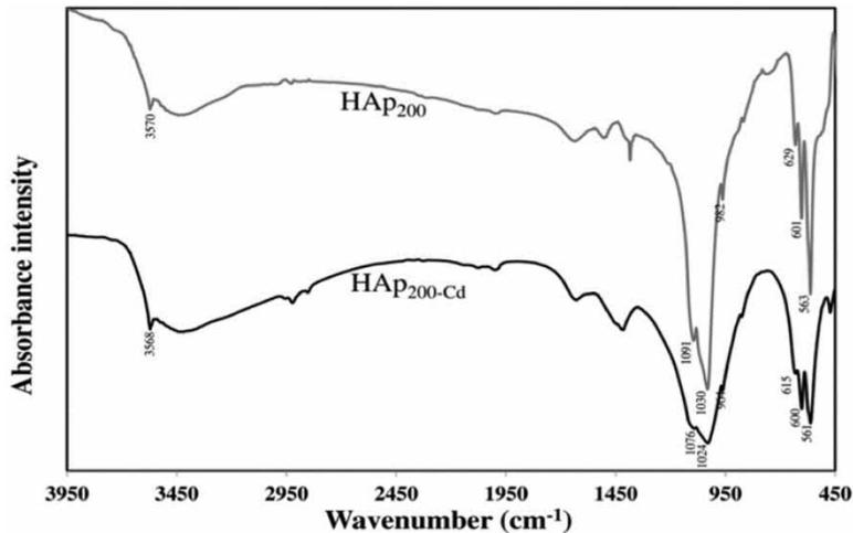
**Figure 13** | IR spectrum of the solid residue with a moderate amount of  $\text{Cd}^{2+}$  uptake ( $q_e = 123.6 \text{ mg g}^{-1}$ ) compared to that of the starting powder.
