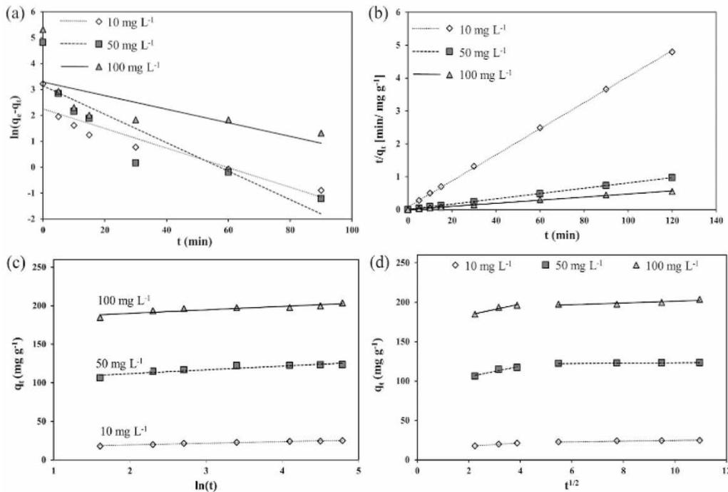
**Figure 8** | Experimental data fitting for adsorption of  $\text{Cd}^{2+}$  ions onto  $\text{HAp}_{200}$  according to the pseudo-first-order (a), pseudo-second-order (b), Elovich (c), and intraparticle diffusion kinetic models (d).
