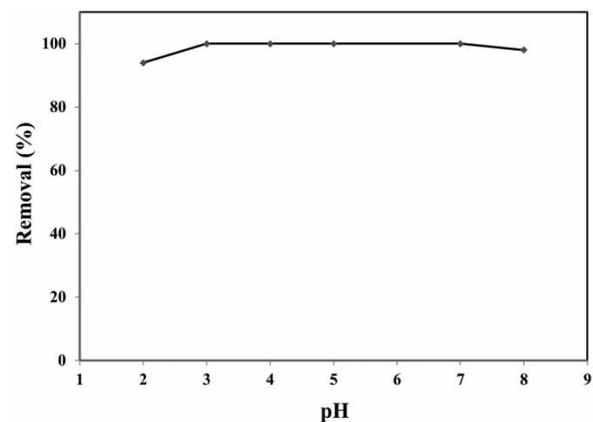
**Figure 4** | Effect of the pH on the removal of Cd<sup>2+</sup> by HAP<sub>200</sub> (Conditions: [Cd<sup>2+</sup>]<sub>0</sub> = 10 mg L<sup>-1</sup>, V = 100 mL, m = 40 mg, t = 120 min).
