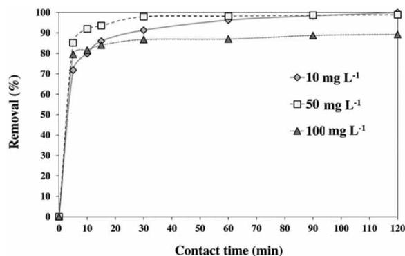
**Figure 6** | Contact time effect on  $\text{Cd}^{2+}$  sorption onto  $\text{HAP}_{200}$  (Conditions:  $[\text{Cd}^{2+}]_0 = 10, 50, \text{ and } 100 \text{ mg L}^{-1}$ ,  $V = 100 \text{ mL}$ ,  $m = 40 \text{ mg}$ ).
