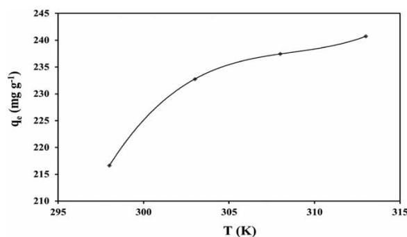
**Figure 7** | Effect of the solution temperature on the uptake of  $\text{Cd}^{2+}$  ions by  $\text{HAP}_{200}$  (Conditions:  $[\text{Cd}^{2+}]_0 = 100 \text{ mg L}^{-1}$ ,  $V = 100 \text{ mL}$ ,  $m = 40 \text{ mg}$ ,  $t = 120 \text{ min}$ ).
