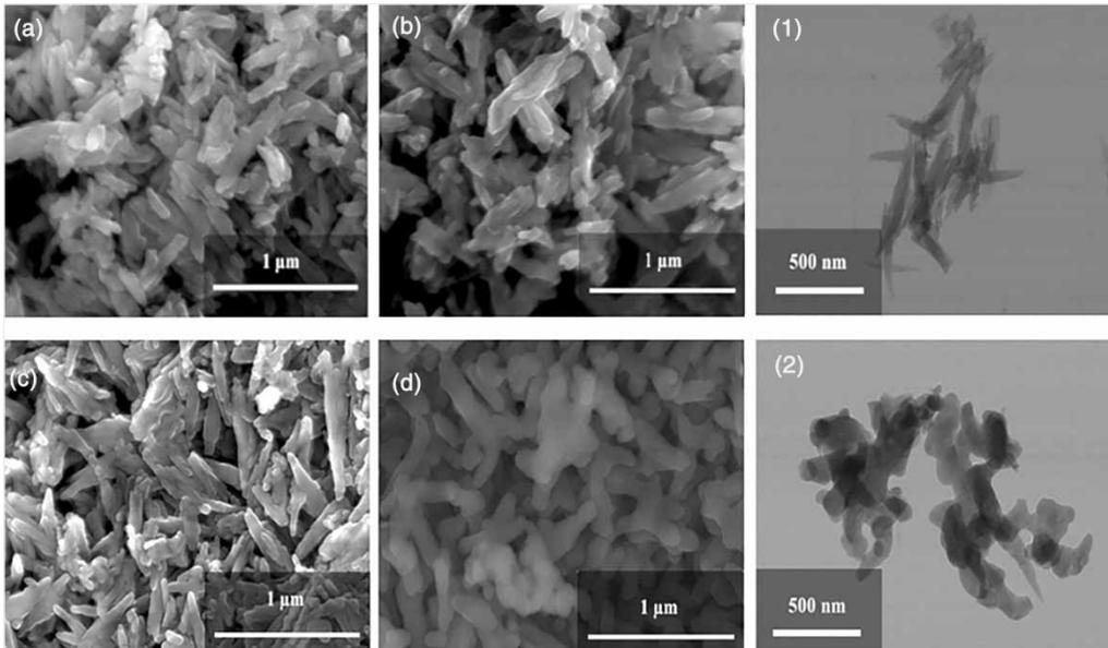
**Figure 11** | SEM micrographs relative to HAP<sub>200</sub> (a), HAP<sub>200</sub>-Cd (b), HAP<sub>800</sub> (c), HAP<sub>800</sub>-Cd (d), and TEM micrographs relative to HAP<sub>200</sub>-Cd (1) and HAP<sub>800</sub>-Cd (2).
