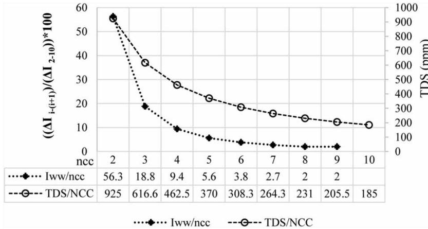
**Figure 2** | Withdrawal water rate and the maximum allowable TDS due to *ncc* variations.
