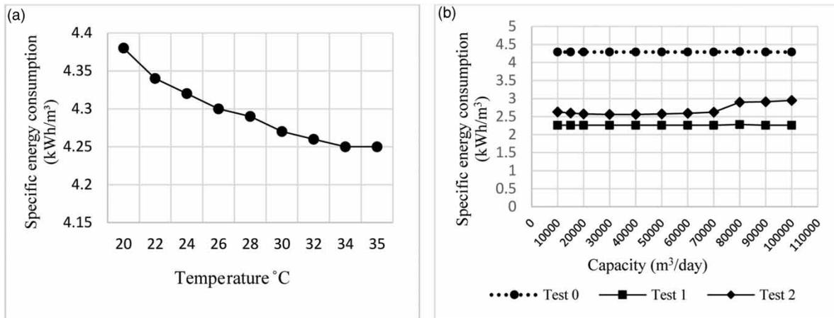
**Figure 3** | (a) The effect of temperature and (b) the effect of capacity on specific energy consumption.
