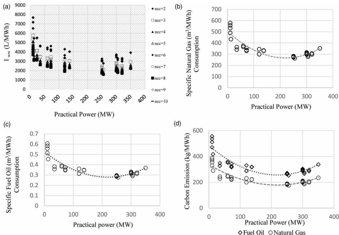
**Figure 4** | The effect of practical power on: (a) specific water withdrawal, (b) specific natural gas consumption, (c) specific fuel oil consumption, and (d) specific carbon emission indicator.
