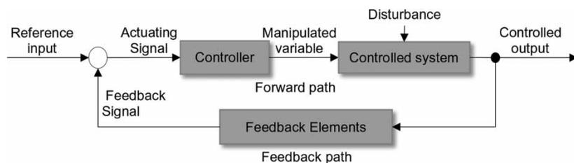
Figure 2 | Closed-loop control (feedback control system).
