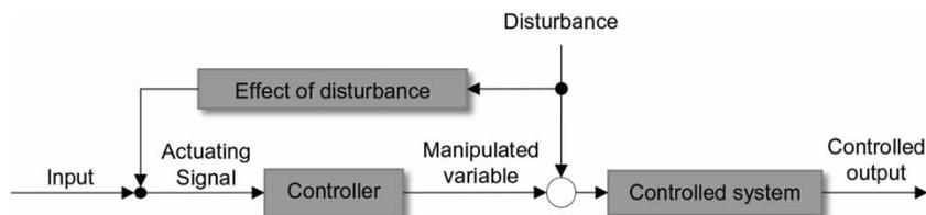
Figure 1 | Feedforward control system.
