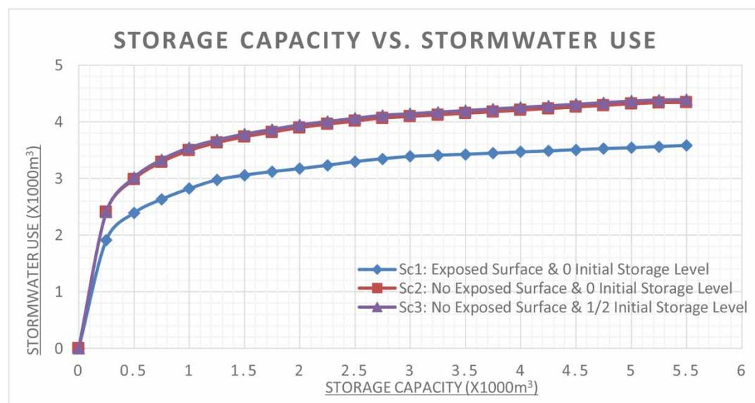
**Figure 6** | Stormwater usage for irrigation and storage capacity.
