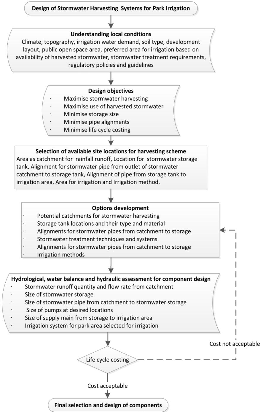
**Figure 1** | Design methodology flowchart for stormwater harvesting scheme.
