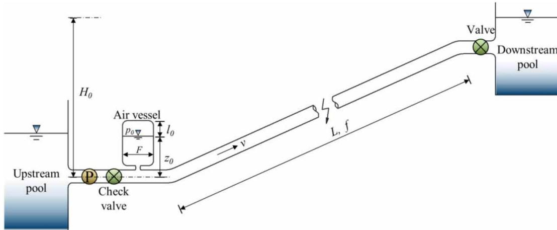
Figure 1 | Layout of the water supply system with air tank protection after the pump.
