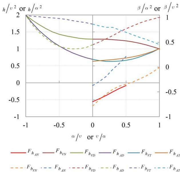
**Figure 4** | Dimensionless-homologous head and torque data for the specific speed  $N_S = 34.8 \text{ rpm}$ : [subscripts A or V =  $h/v^2$  vs  $\alpha/v$  or  $h/\alpha^2$  vs  $v/\alpha$ , respectively; and subscripts N, D, or T = normal, energy dissipation, or turbine operation zones, respectively].
