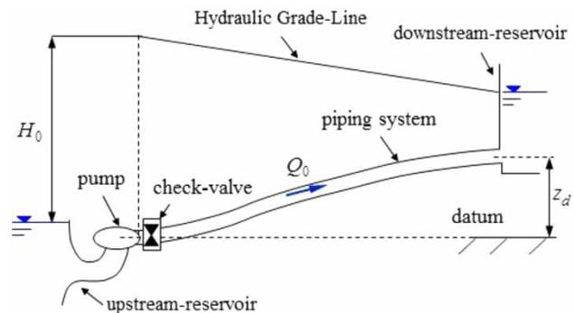
**Figure 6** | Hydraulic system layout.
