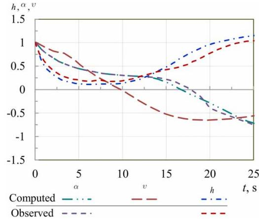
**Figure 5** | Comparison of computed and observed dimensionless pressure-head, velocity, and speed signals.
