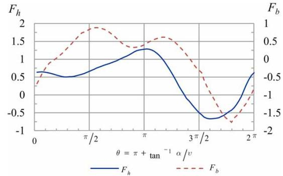
**Figure 7** | Suter's curves for the specific speed  $N_s = 25$  rpm.
