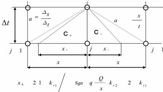
Figure 1 | Characteristics lines in the (x – t) plane, for the Ramos *et al.* formulation.
