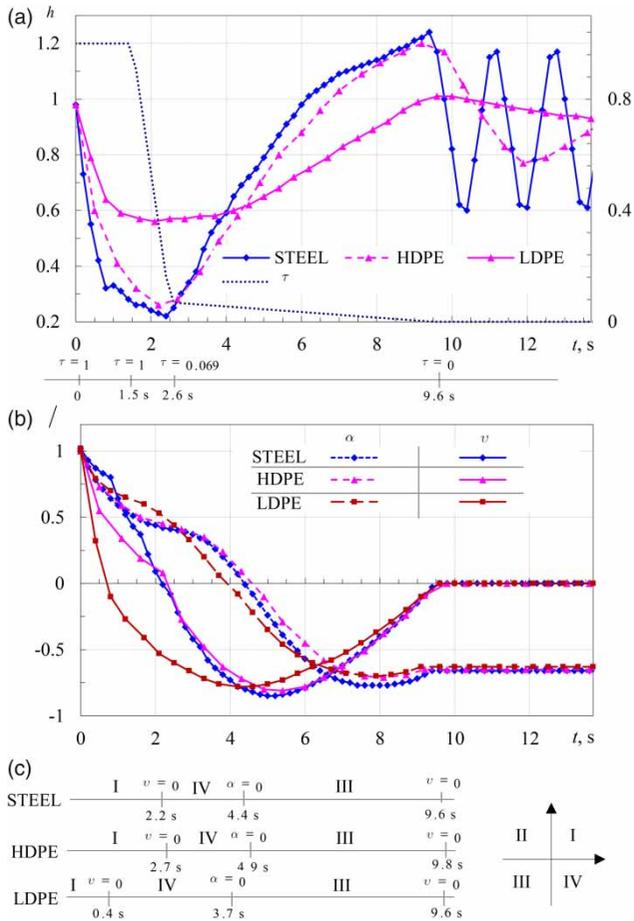
**Figure 8** | Dimensionless (a) pressure-head and valve position; (b) velocity and speed; and (c) zones of pump operation (I = normal, II = reversed speed dissipation, III = turbine, and IV = dissipation zones).
