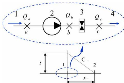
Figure 2 | Schematic illustration of the pump and its control valve at the upstream extremity (node 1) [(1,4) flow; (2) pump; (3) check-valve].
