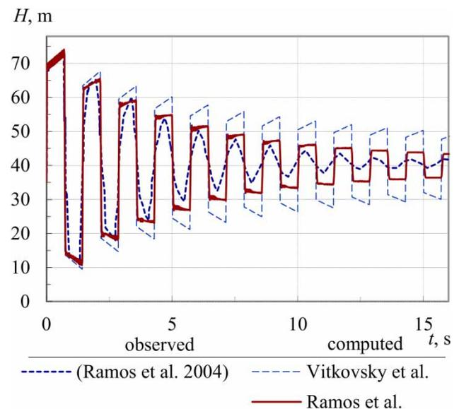
**Figure 3** | Comparison of pressure-head signals obtained from experimental observations and numerical computations using the Vitkovsky *et al.* ( $k_v = 0.03$ ) or Ramos *et al.* ( $k_{r1} = 0.003/k_{r2} = 0.04$ ) formulations.
