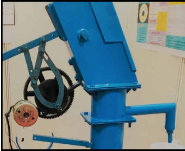
**Figure 7** | Hand pump fitted with gear wheels and dynamo.
