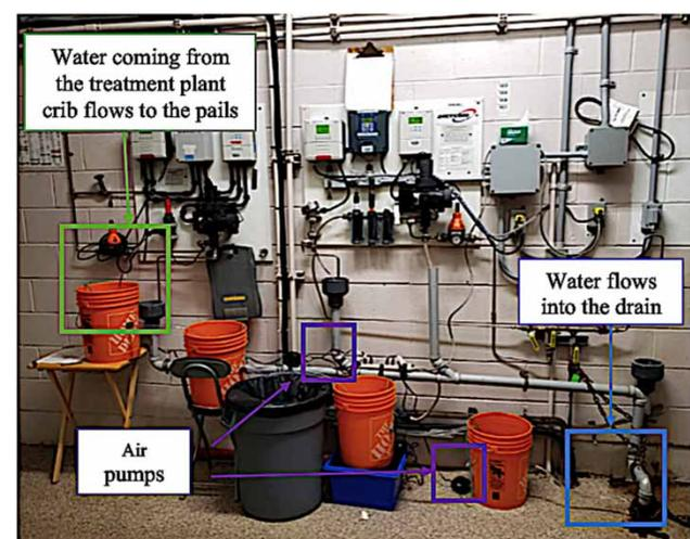
**Figure 1** | Acclimatization system for adult mussels at the AP Kennedy Water Treatment Plant.
