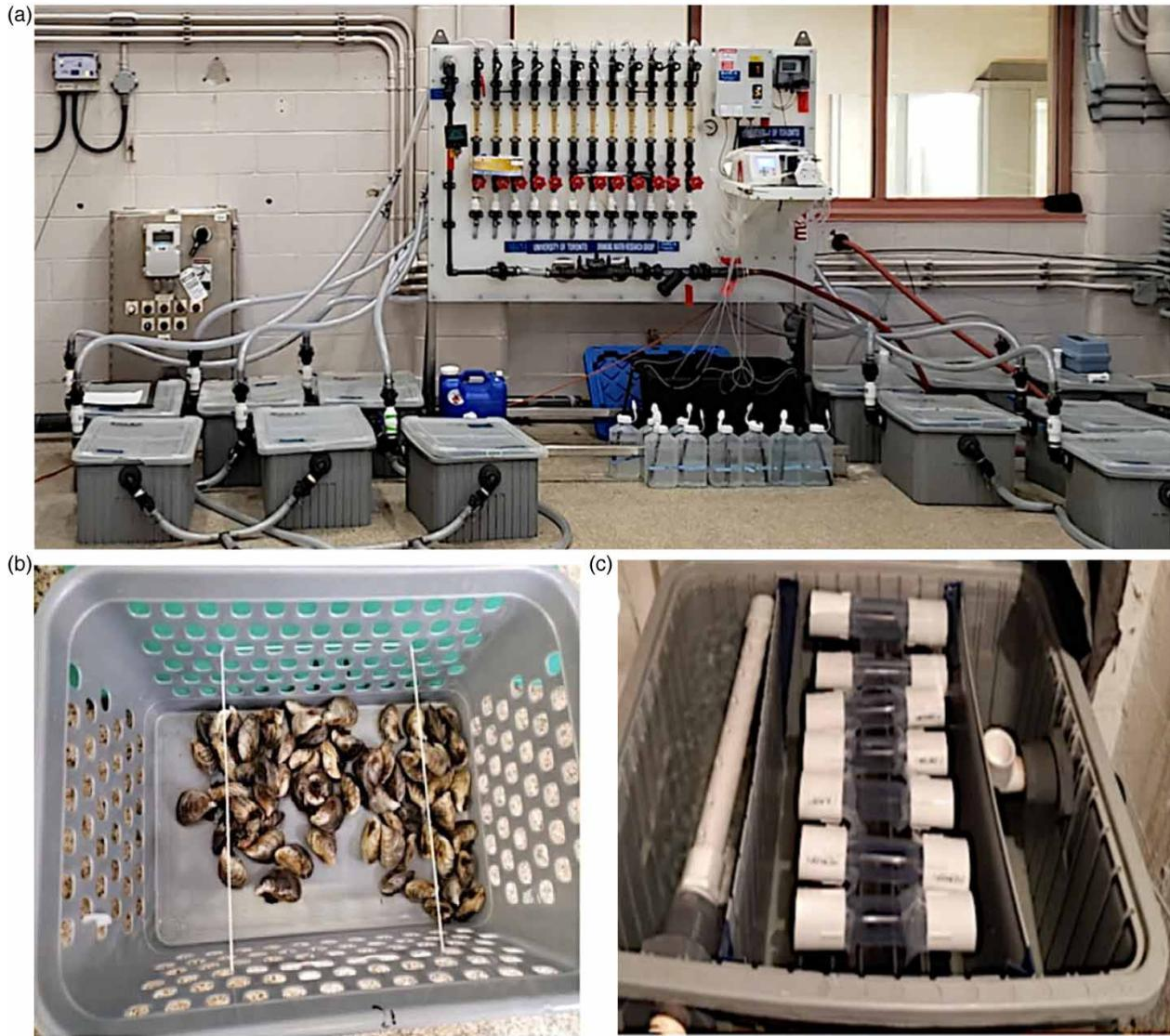
**Figure 2** | Apparatus used for the flow-through experiments: (a) pilot-scale dosing system and bioboxes, (b) bioassay tray for adult mussels, and (c) biotubes for veligers.
