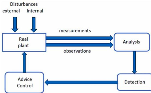
**Figure 3** | A monitoring system is based on analysis of measurements and observations. A fault or failure can often be detected automatically. Based on the result, some advice or operator support can be given, and a control action can take place.
