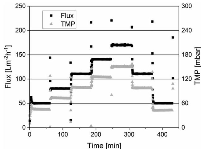
**Figure 3** | TMP development during the stepping-flux method for 20 g/L KM at  $\Delta t = 60$  min from 50 to 170 L m<sup>-2</sup> h<sup>-1</sup> by  $\Delta J = 30$  L m<sup>-2</sup> h<sup>-1</sup>.
