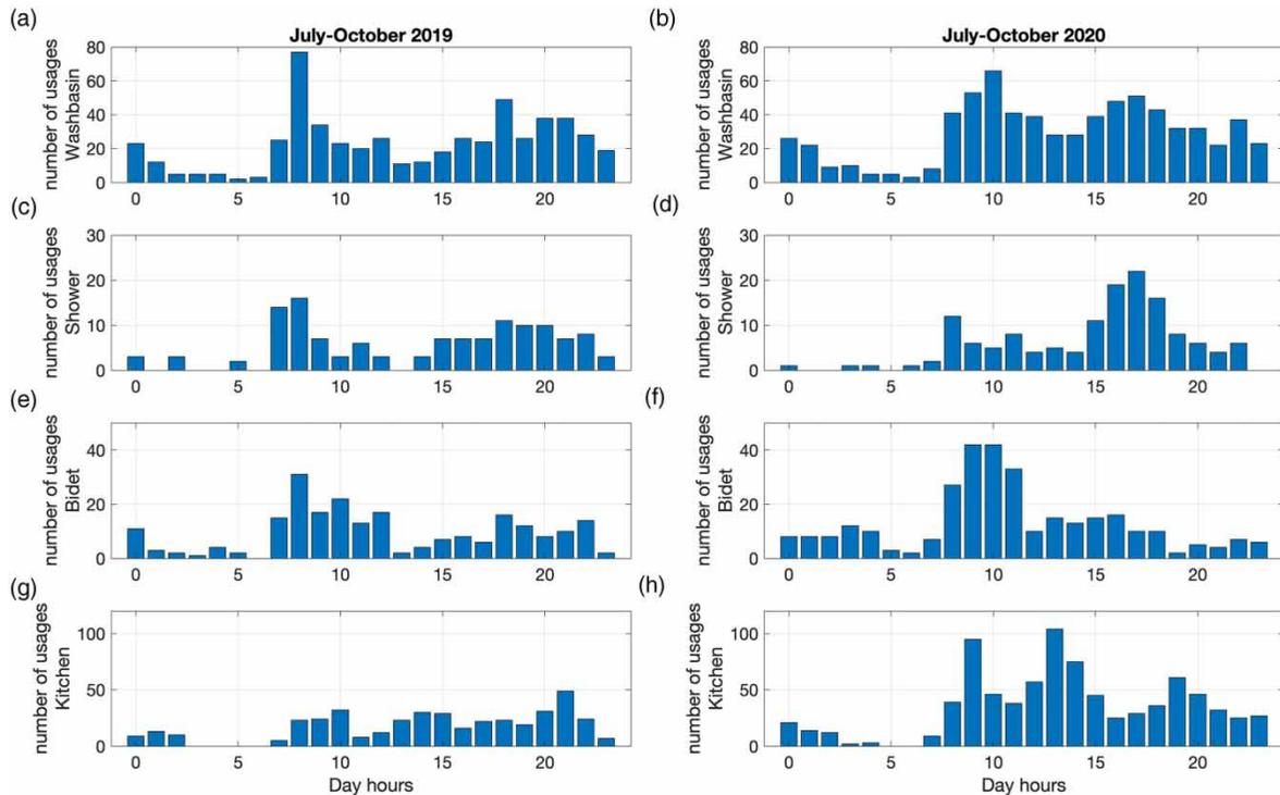
**Figure 3** | (a)–(h) Number of users during day hours for different fixtures evaluated on the same 4 months of measurements (July–October) of different years 2019 and 2020: (a) Washbasin 2019, (b) Washbasin 2020, (c) Bidet 2019, (d) Bidet 2020, (e) Shower 2019, (f) Shower 2020, (g) Kitchen 2019, and (h) Kitchen 2020.
