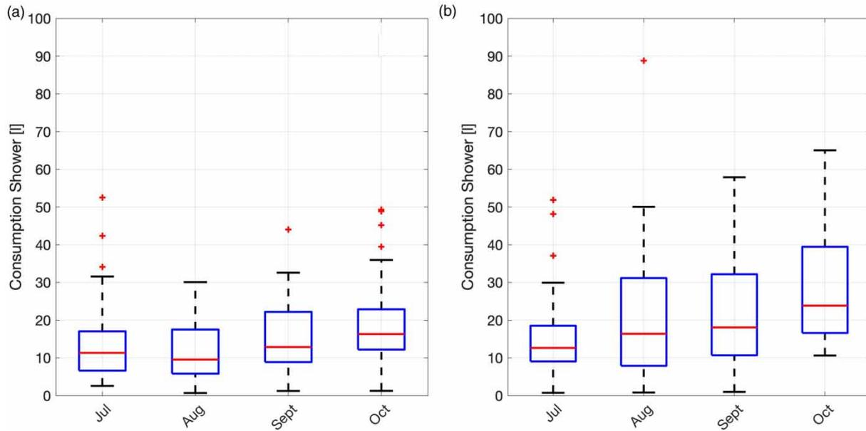
**Figure 1** | The figure shows for one of the fixtures (Shower). The water consumption evaluated from July to October in both 2019 (a) and 2020 (b). Please refer to the online version of this paper to see this figure in colour: <http://dx.doi.10.2166/aqua.2021.088>.
