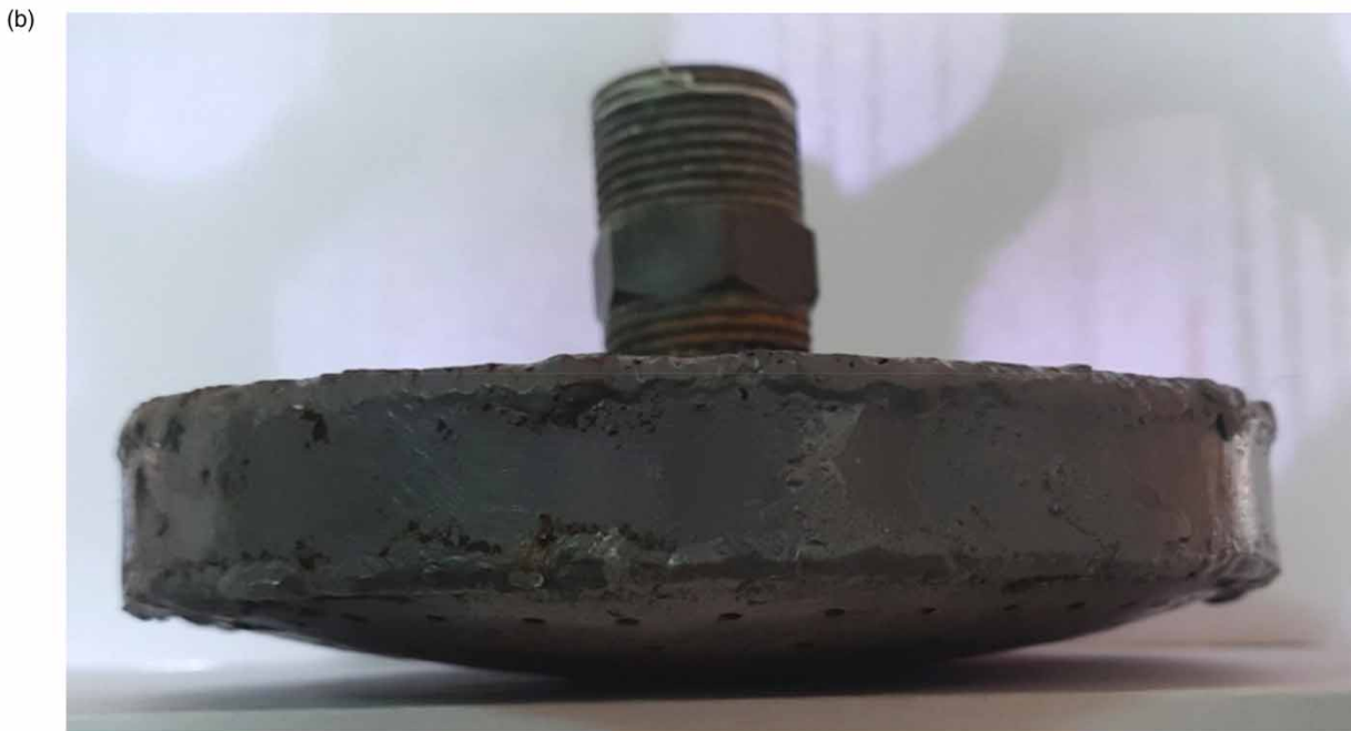
Figure 2 | (a) CAD model and (b) fabricated shower.
