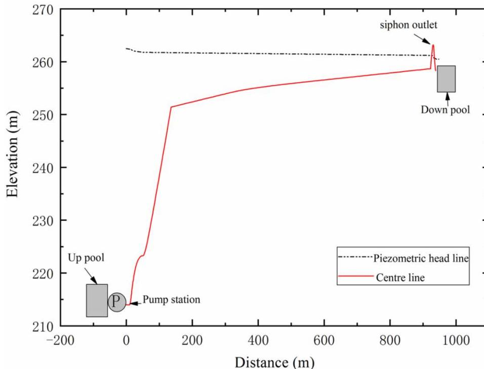
**Figure 3** | Pipe centerline, piezometric headline and schematic diagram of the water supply project.
