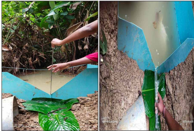
Figure 5 | Discharge determination using V-notch.
