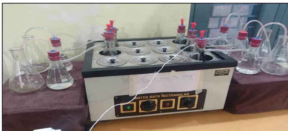
Figure 2 | Laboratory anaerobic batch digestion setup.
