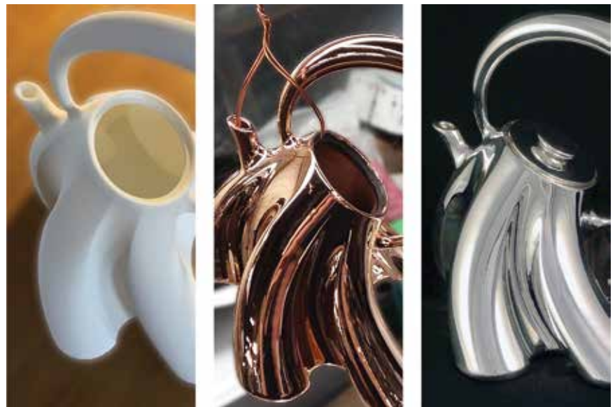
Fig. 4. Details of the teapot (from left to right) in SLS nylon polyamide, copper electroform and silver plate. (Photo: © Courtney Starrett)
