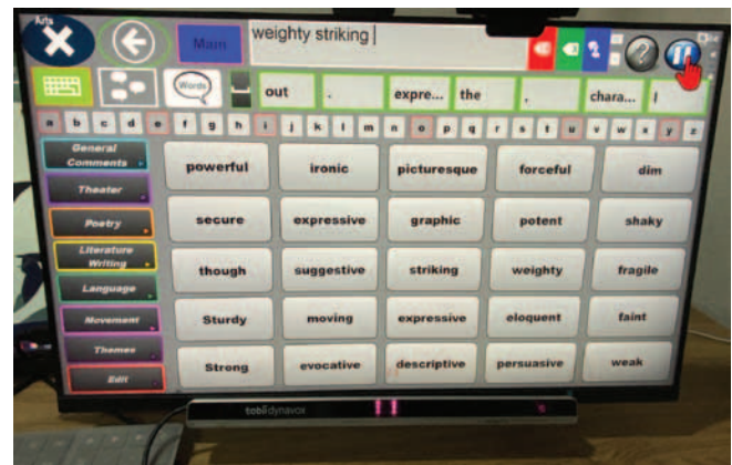
Fig. 3. This is the Communicator page that Ysolde opened to respond to the first part of this article. Notice the marks on the button that says "descriptive": these are the marks of Ysolde's eyes picked up by the Tobii eye-gaze tracker, its pulsed infrared light (IR) glowing as two dotted lines below the screen. The words selected show up at the top, where the cursor is. These are voiced by the computer. (Usually, the selected words need to be manually reset; otherwise the computer can begin a run-on sentence of all previous selections.) (Photo © Marina Tsaplina)
