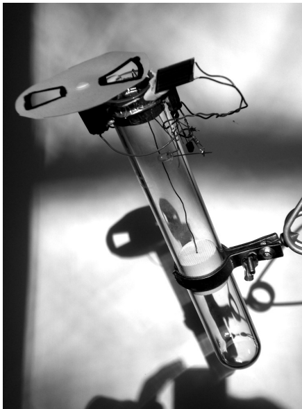
Fig. 5. A hybrid automaton combining singing tube (generator) and a simple "solarengine" photovoltaic circuit patented by Mark Tilden (actuator). (Photo © M. Duffey) The solarengine rotates a slotted cover over the tube to control on/off cycling. It can also be used to vary pitch.
