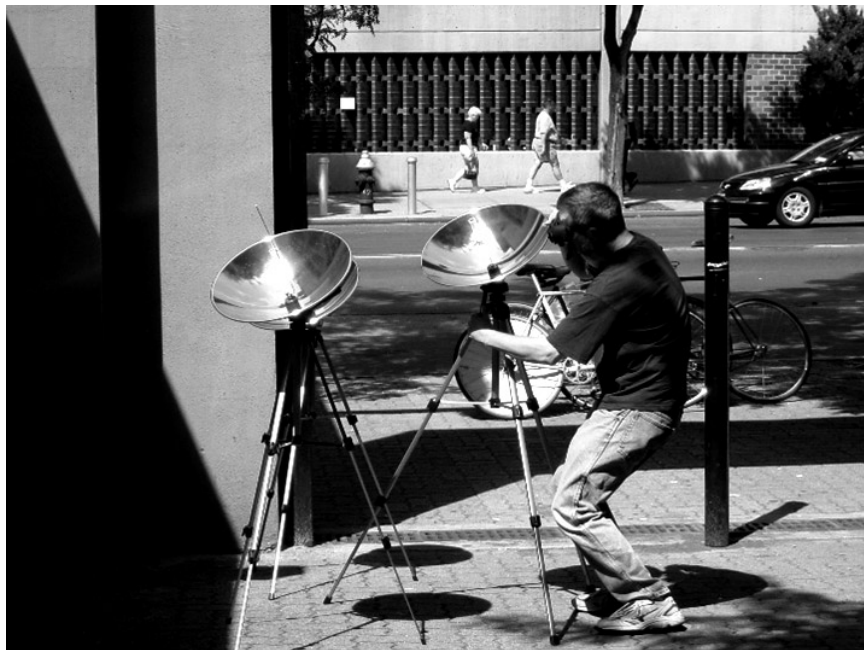
Fig. 2. A memnonium prototype demonstrated at The Tank in New York City, July 2003. (Photo © M. Duffey) Three parabolic solar concentrators have their focal areas aligned with “singing tubes” for a chord triad. Note the need for eye protection.
