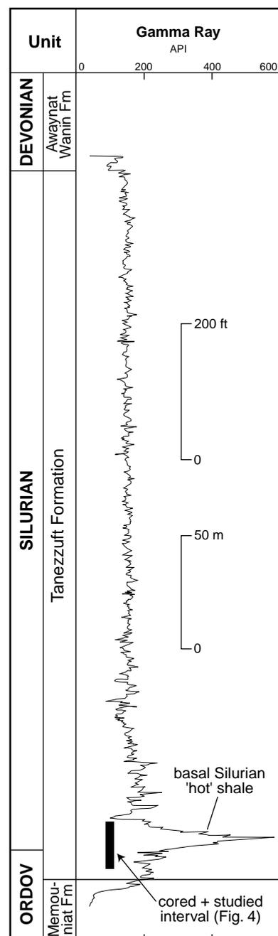
**Figure 2: Total gamma-ray log of well E1-NC174. Latest Ordovician-early Silurian Tanezzuft Shale Formation with the basal radioactive, organic-rich 'hot' shale, overlying Ordovician sandstones of the Memouni at Formation (modified after Lüning et al., 2000).**
