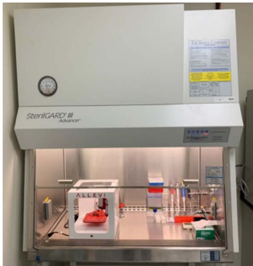
**Fig. 4 Allevi 2 bioprinter in a biosafety cabinet**
