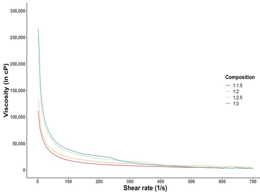
**Fig. 3 Relationship between viscosity and shear rate**
