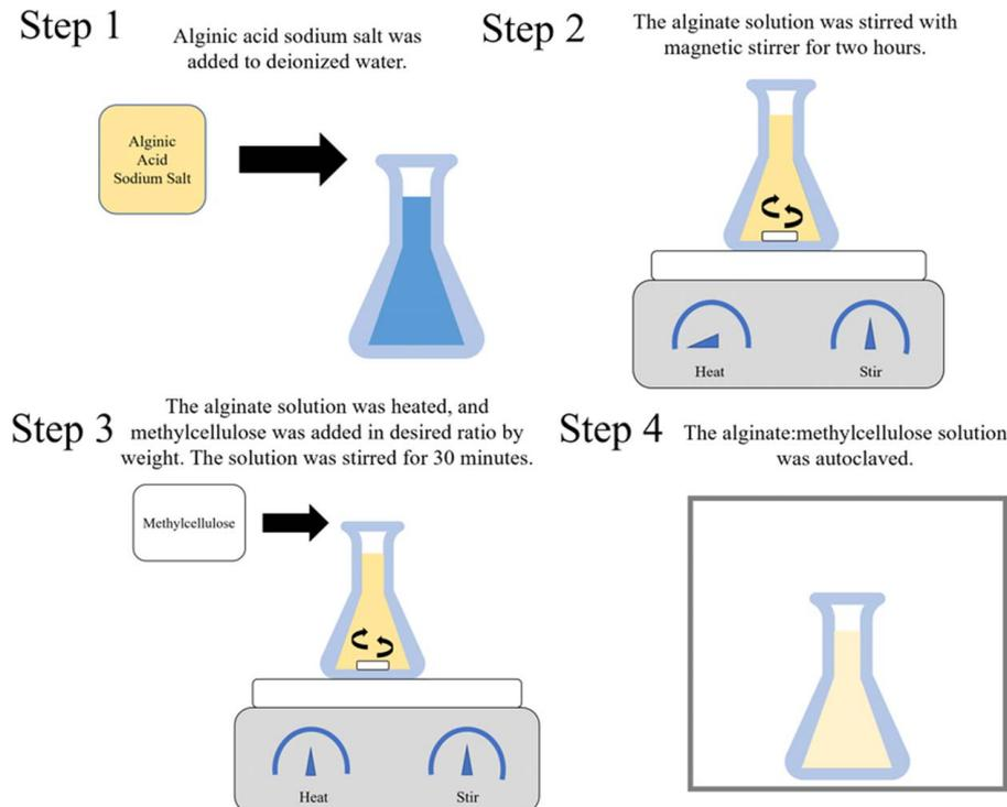
**Fig. 2 Procedure for bioink synthesis**
