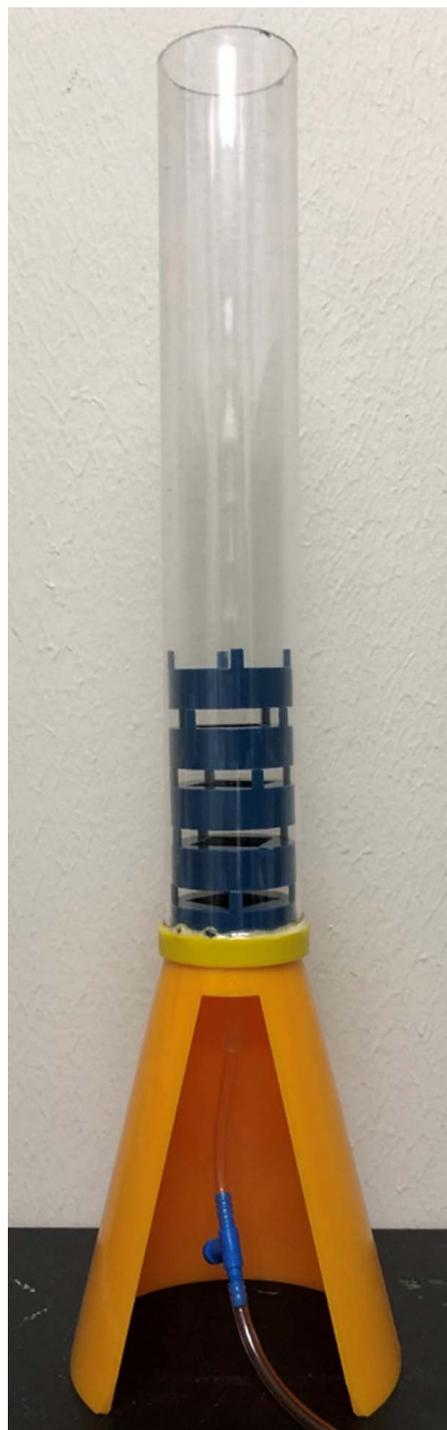
**Fig. 4 Filtration chamber**
