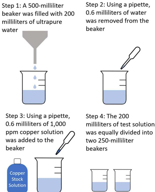
Fig. 6 Test solution preparation
