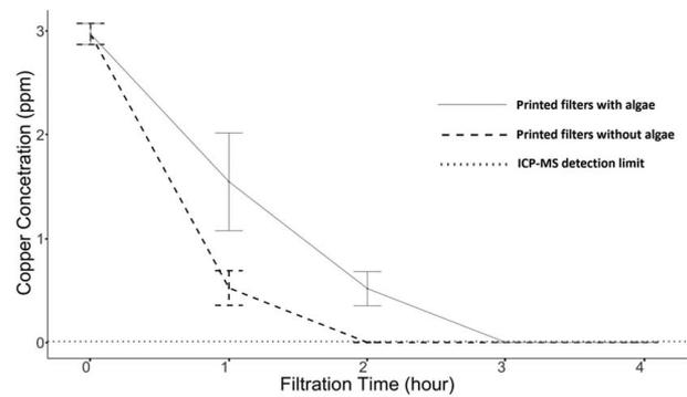
**Fig. 8 Relationship between copper concentration and filtration time**
