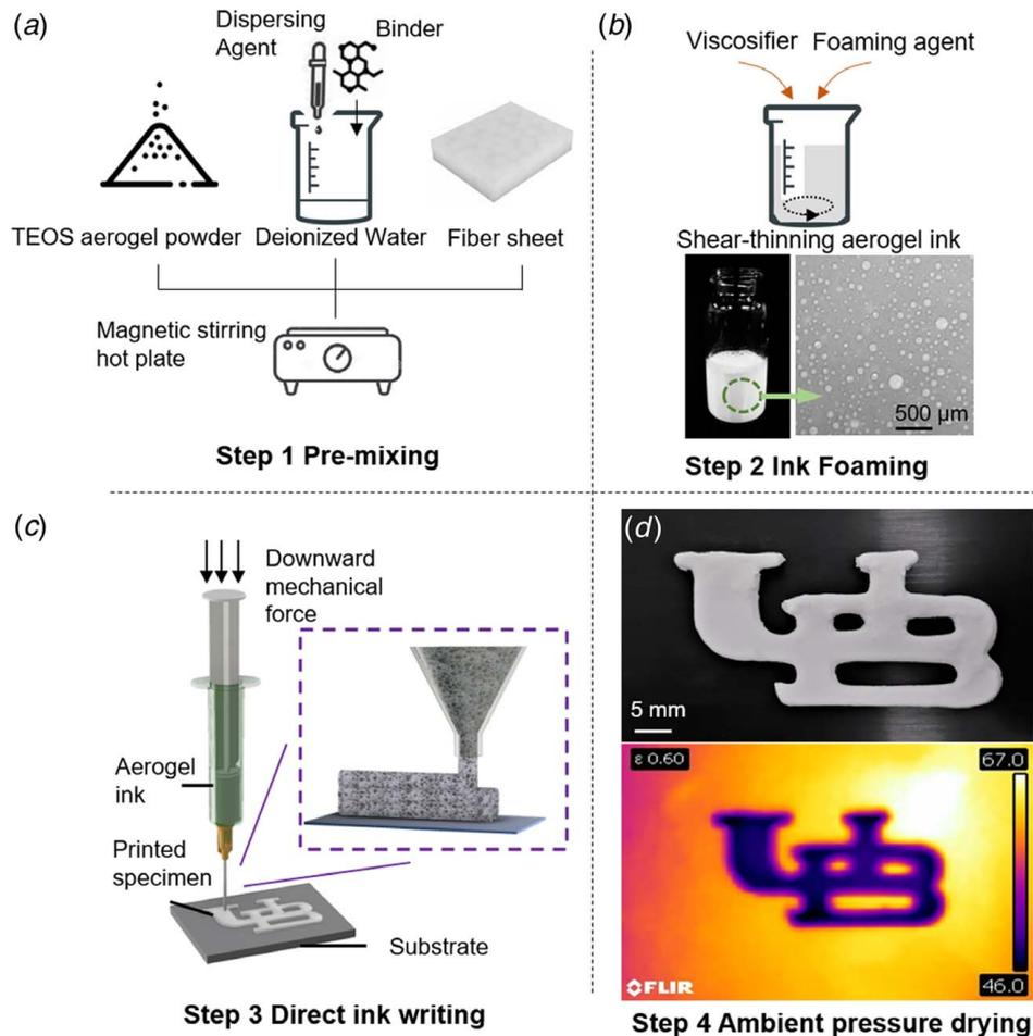
**Fig. 1** Direct ink writing of silica aerogel insulation material. (a) The recipe and pre-mixing step of preparing aerogel ink. (b) The presence of additives in the ink ensures its printability. The gaseous bubbles are uniformly distributed in the ink. (c) Schematic diagram of the direct ink writing process. (d) The aerogel printed object with a UB logo geometry and its infrared image showing the thermal insulation property.
