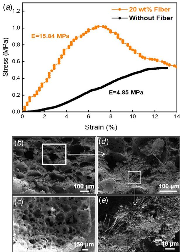
**Fig. 5 Mechanical properties characterization and microstructure characterization. (a) Stress-Strain curves for specimens without fiber and with 20 wt% fiber content. (b) and (c) are SEM images to show the internal porous structure. (d) and (e) show the bonding between fiber and aerogel skeleton.**
