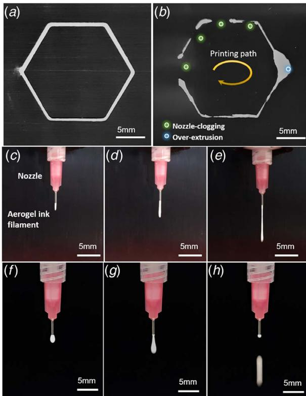
**Fig. 2** Characterization of the aerogel ink. (a) A hexagon contour written by aerogel ink with suitable rheology. (b) Unfavorable ink printability. (c)–(e) The shear-thinning behavior of the aerogel ink. (f)–(h) The ink without shear-thinning behavior cannot form continuous and uniform filament.
