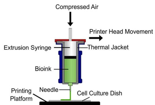
**Fig. 1** Illustration of extrusion-based bioprinting process
