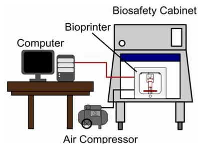
Fig. 3 Illustration of printing experimental setup
