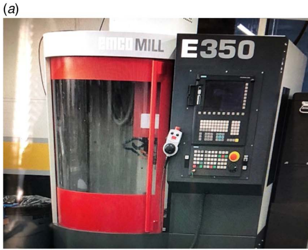
Fig. 1 (a) EMCOMILL E350 three-axis vertical CNC mill, equipped with (b) Siemens 828D controller
