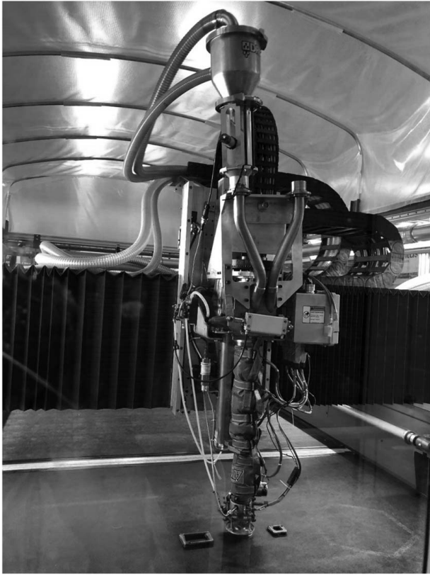
Fig. 2 BAAM extruder during a print
